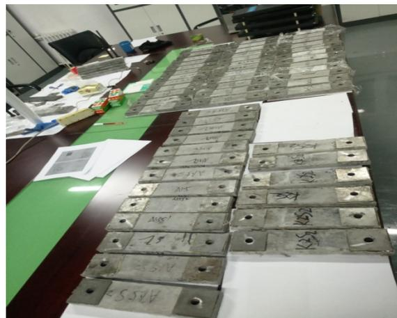
**Figure 3.** Specimens with the end reinforcement.
