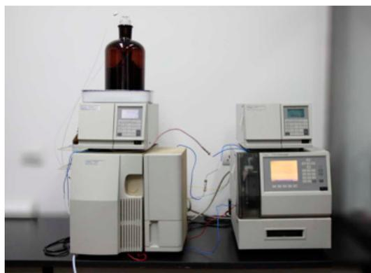
**Figure 2.** Gel permeation chromatography (GPC) system.
