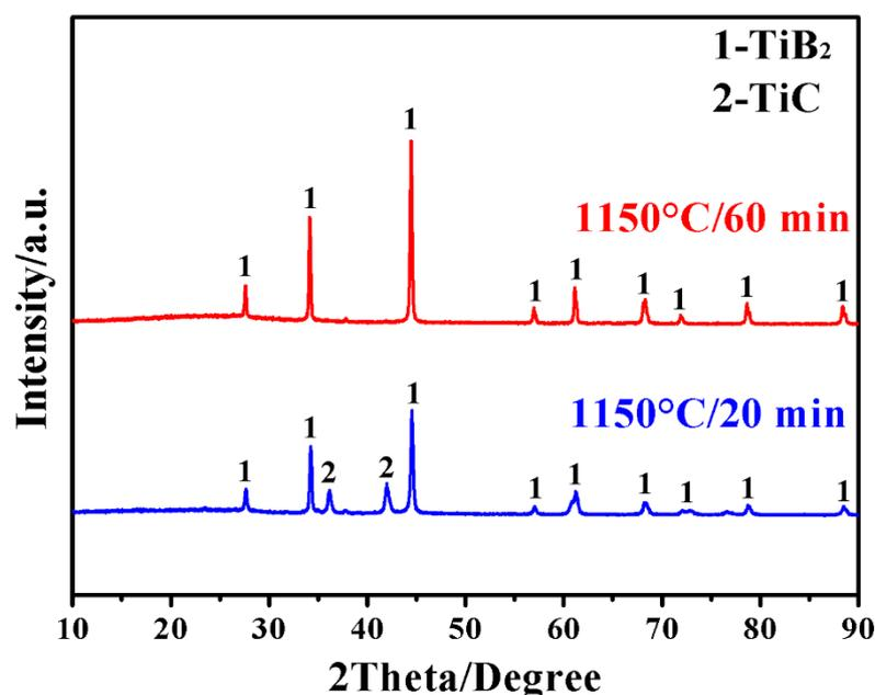
**Figure 1.** Phase formation in samples prepared by MSM-BCTR at 1150 °C for respectively 20 and 60 min.
