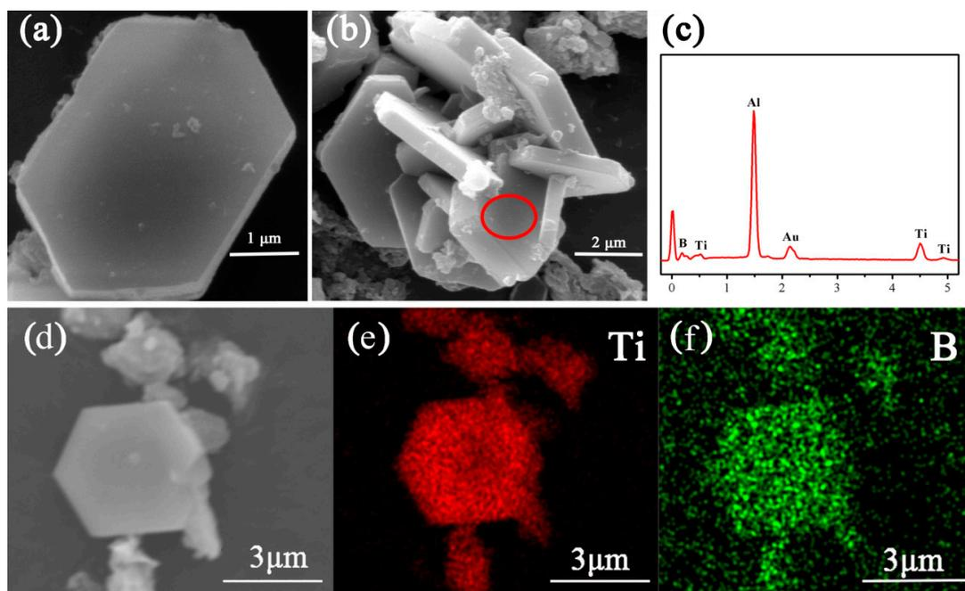
**Figure 5.** SEM images of (a) monodispersed  $\text{TiB}_2$  microplatelet and (b) interlaced  $\text{TiB}_2$  microplatelets, (c) corresponding EDS results of  $\text{TiB}_2$  microplatelets, (d) a lower magnification SEM image with EDS mappings of (e) Ti element and (f) B element prepared *via* MSM-BCTR at  $1200^\circ\text{C}$  for 20 min. (Au and Al peaks in Figure 5b were from the gold coating and aluminum foil used for enhancing electrical conductivity of the powder sample.)
