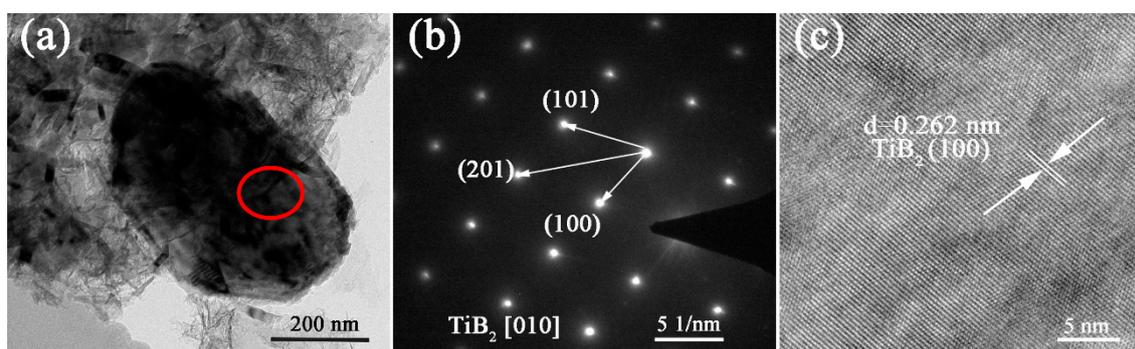
**Figure 6.** (a) Low-magnification TEM image and (b) SAED pattern of a representative  $\text{TiB}_2$  microplatelet in the sample prepared *via* MSM-BCTR at 1200 °C for 20 min, and (c) high-resolution TEM image taken in the area defined by the red circle in (a).
