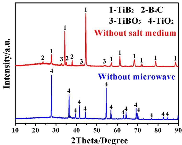
**Figure 3.** Phase formation in MSM-BCTR samples resultant from 20 min firing at 1200 °C, using solely microwave heating or molten-salt medium.
