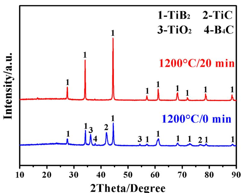
**Figure 2.** Phase formation in samples after MSM-BCTR treatments at 1200 °C for 0 and 20 min, respectively.
