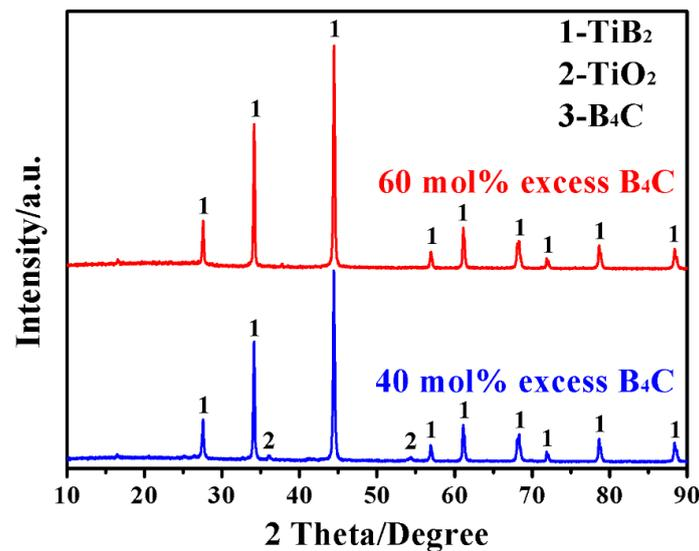
**Figure 4.** XRD patterns of samples containing initially 40 and 60 mol% excessive  $\text{B}_4\text{C}$ , after MSM-BCTR treatments at  $1200^\circ\text{C}$  for 20 min.
