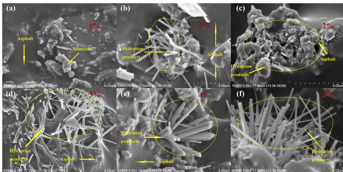
Figure 5. Microstructure of mortar with different contents of cement. (a) Without cement. (b) With 1% cement. (c) With 2% cement. (d) With 3% cement. (e) With 4% cement. (f) With 5% cement.
