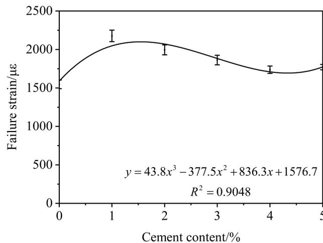
**Figure 3.** Results of three-point bending test.
