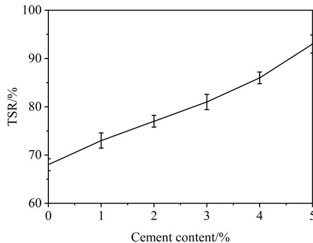
Figure 4. Results of moisture susceptibility test.
