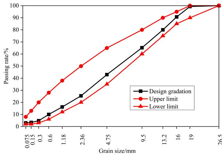
Figure 1. Grading curve of CRME.
