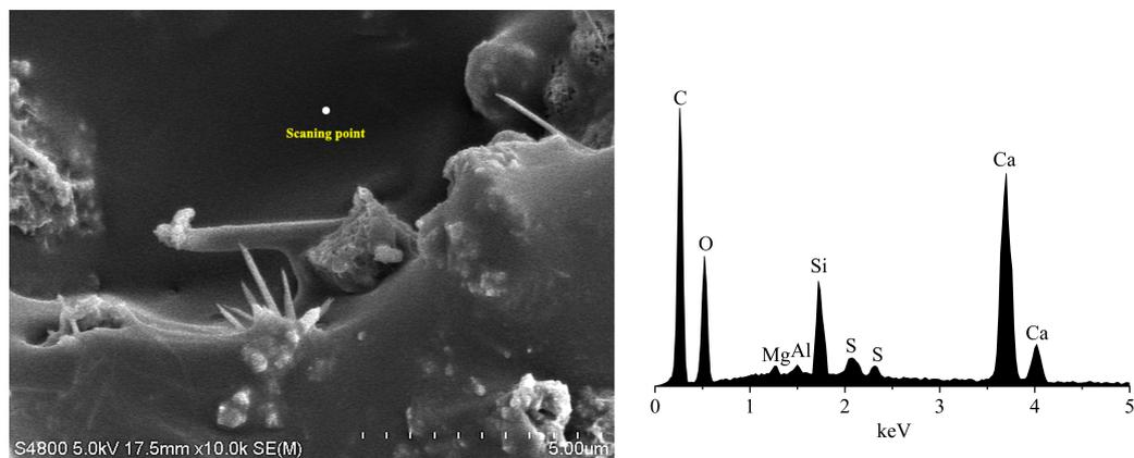
Figure 8. Chemical composition of CRME with 2% cement.
