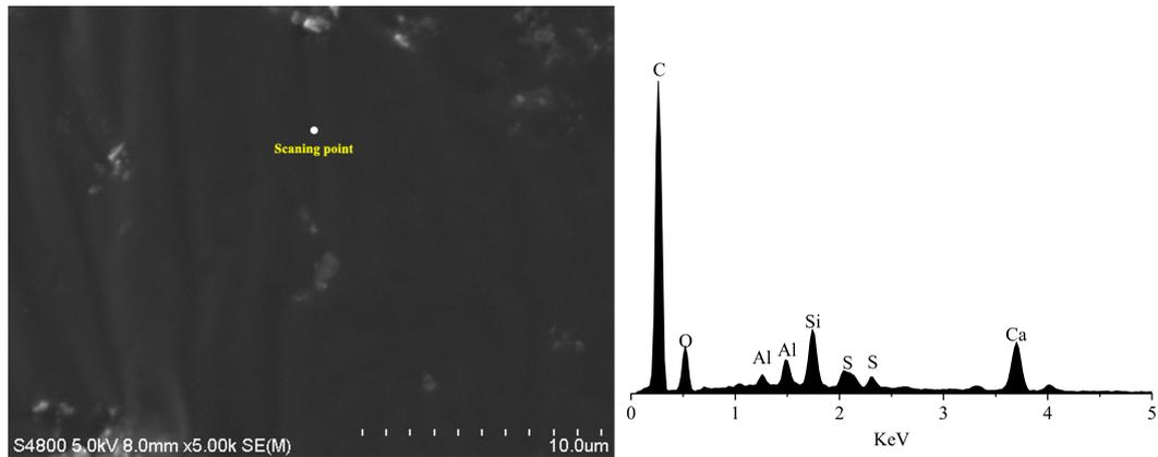
Figure 7. Chemical composition of CRME without cement.
