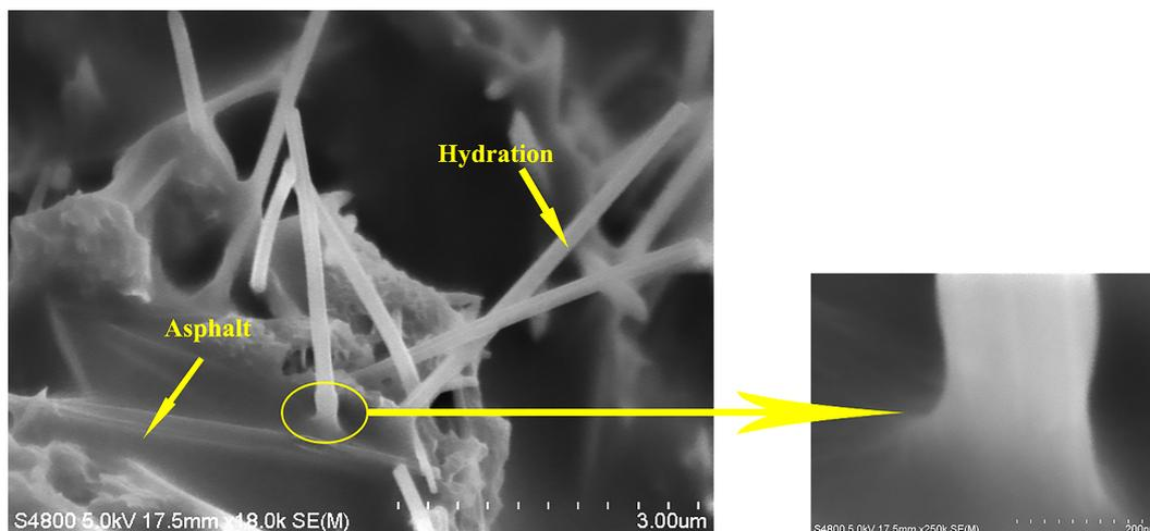
**Figure 6.** The adhesive state between asphalt membrane and hydration products.
