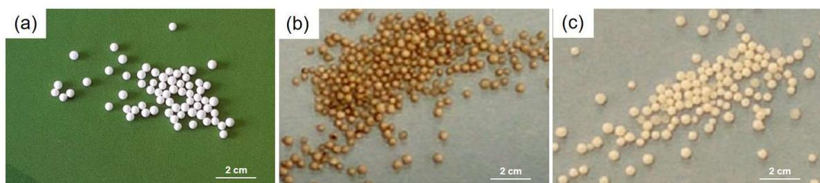
**Figure 3.** Color and size of (a) PLGA microspheres, (b) PLGA@PDA microspheres and (c) PLGA@PDA/PEI microspheres.
