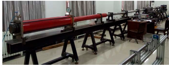
Figure 1. Split Hopkinson pressure bar (SHPB) equipment.
