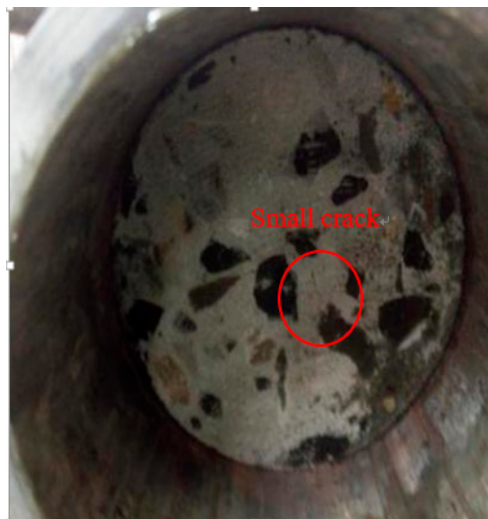
Figure 5. Picture of concrete specimen under impact compression with passive confining pressure (18.36 m/s, 600 °C).
