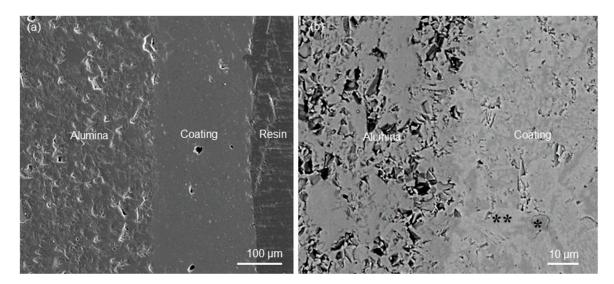
**Figure 3.** Analysis of the coating cross section: (a) SEM micrograph in "secondary" mode  $(400\times)$  and (b) high-magnification detail  $(2500\times)$  inspected in back-scattering mode showing the interface between coating and alumina as well as the coating microstructure (glass–ceramic nature); the white areas (\*\*) correspond to the wollastonite crystals, while the dark zones (\*) correspond to the residual glassy phase.
