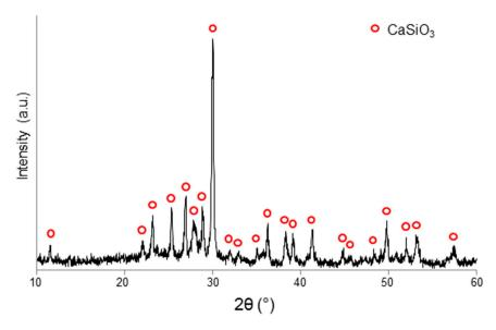
**Figure 2.** XRD pattern of a sintered coating (1000 °C/3 h).
