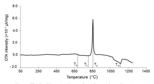
Figure 1. DTA plot of the starting glass powder used to manufacture the coatings.
