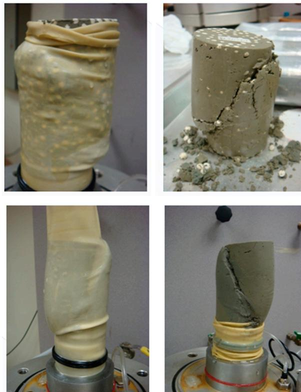
**Figure 9.** Shear failure for the lower E/S ratio.
