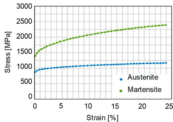
Figure 7. Flow stress curves of austenite and martensite phase.
