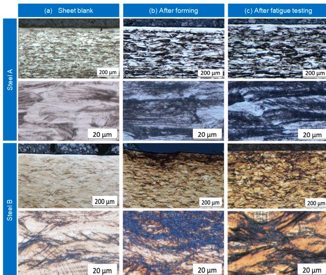
**Figure 14.** Micro-graphs of steel A and steel B cross-sections: (a) Sheet blank, (b) after forming, (c) after fatigue testing.
