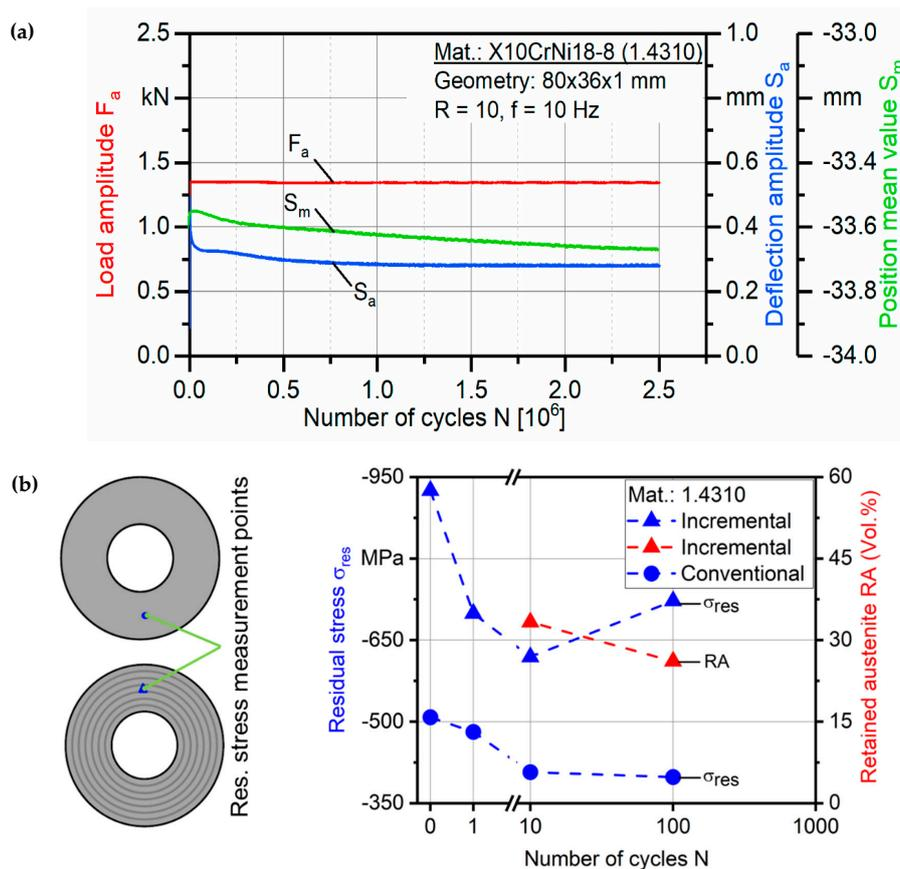
**Figure 13.** (a) Fatigue life investigation with a constant load amplitude for an incrementally formed disc spring of steel A. (b) Stability of the residual stresses in the first 100 loading cycles for steel A.
