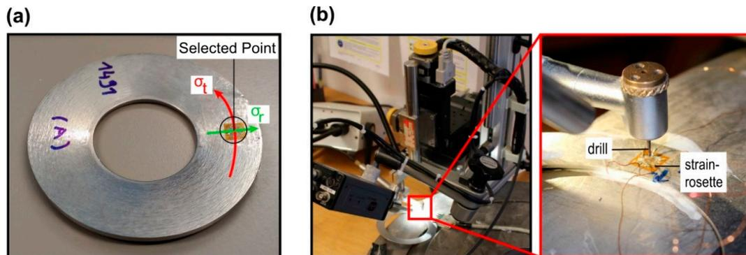
**Figure 3.** (a) Selected point for the measurement of the residual stresses, and (b) experimental set-up of the hole drilling method.
