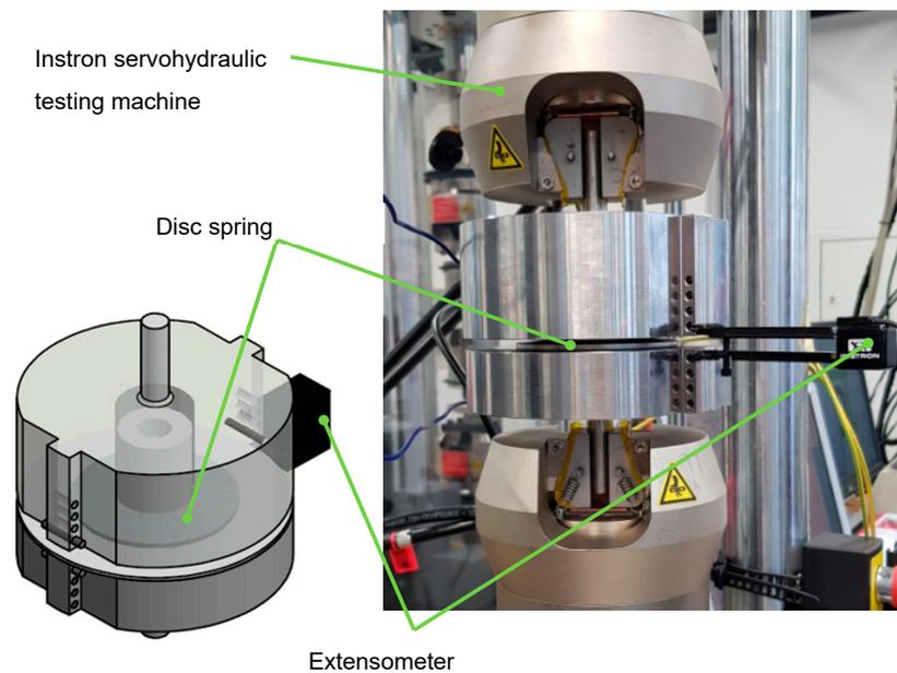
**Figure 5.** Experimental set-up for the quasi-static and cyclic testing of the disc springs.
