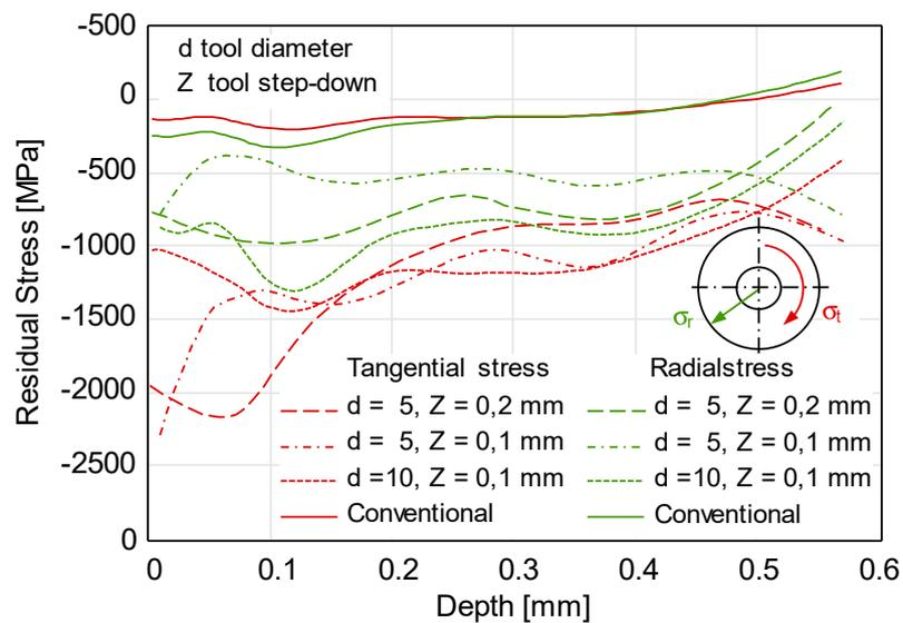
**Figure 10.** Residual stresses measured by the hole drilling method in conventional and in incrementally formed disc springs from steel A under varying process parameters.
