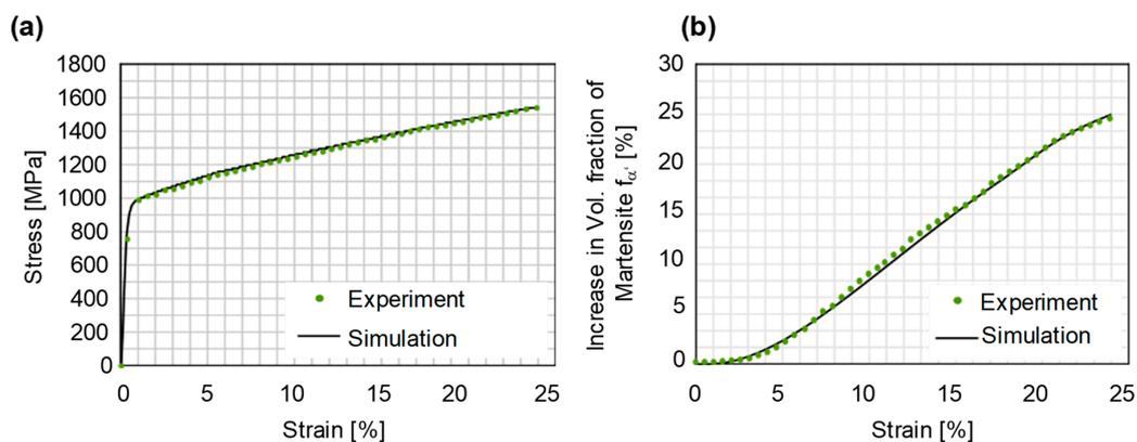
Figure 8. Comparison of experimental and optimized numerical curves: (a) Stress-strain, (b) evolution of the martensite content as a function of the plastic strain.
