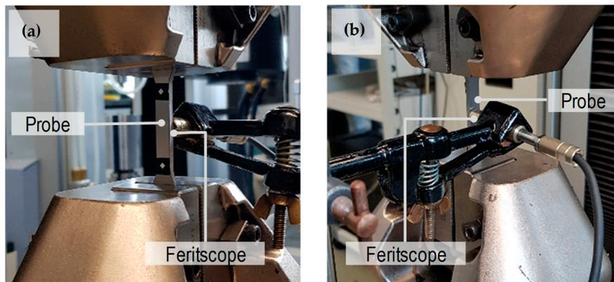
**Figure 6.** (a) Tensile test with a probe for in-site ferromagnetic content measurements (b) stress-strain response and evolution of martensite content as a function of plastic strain.
