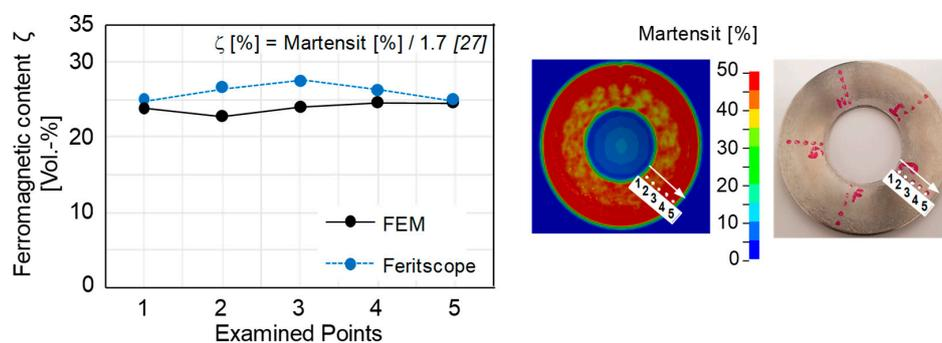
**Figure 15.** Comparison of the experimental and numerical ferromagnetic content measured at five locations on the bottom surface of the disc spring.
