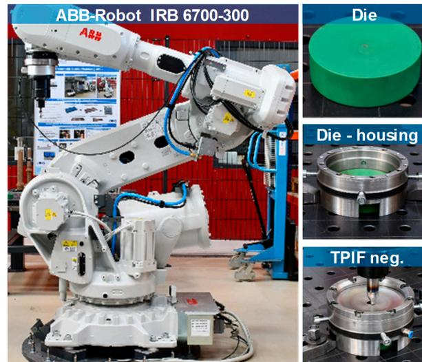
**Figure 2.** Experimental set-up of two-point incremental forming (TPIF) with a negative die using ABB-Robotic arm.
