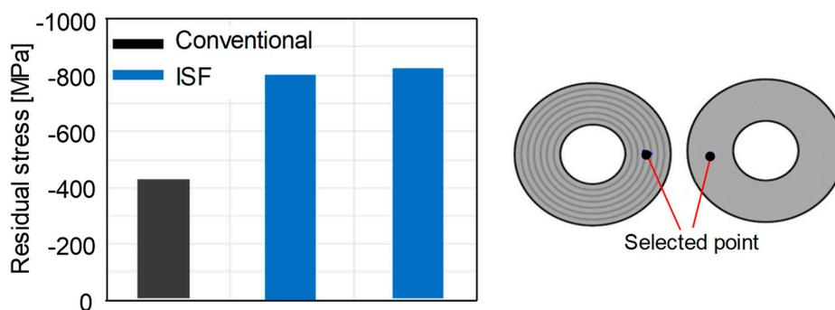
**Figure 11.** Repeatability of the residual stresses measured by X-ray diffraction (XRD) in conventional and incrementally formed disc springs from steel B under the same set of process parameters.
