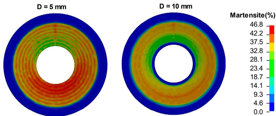
**Figure 17.** Comparison of the martensite content on the bottom surface of the disc springs for different tool diameters.
