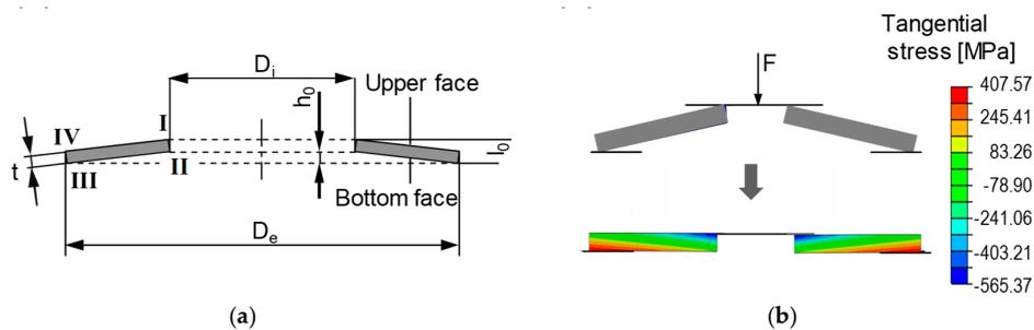
**Figure 1.** (a) The schematic of a conventional disc spring geometry. (b) Development of the stresses in disc springs under normal loading condition.
