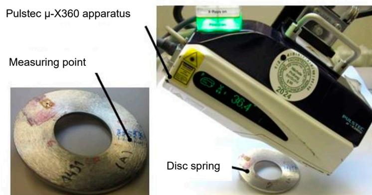
**Figure 4.** Experimental setup for the measurement of the residual stresses in disc springs by portable residual stress analyzer.
