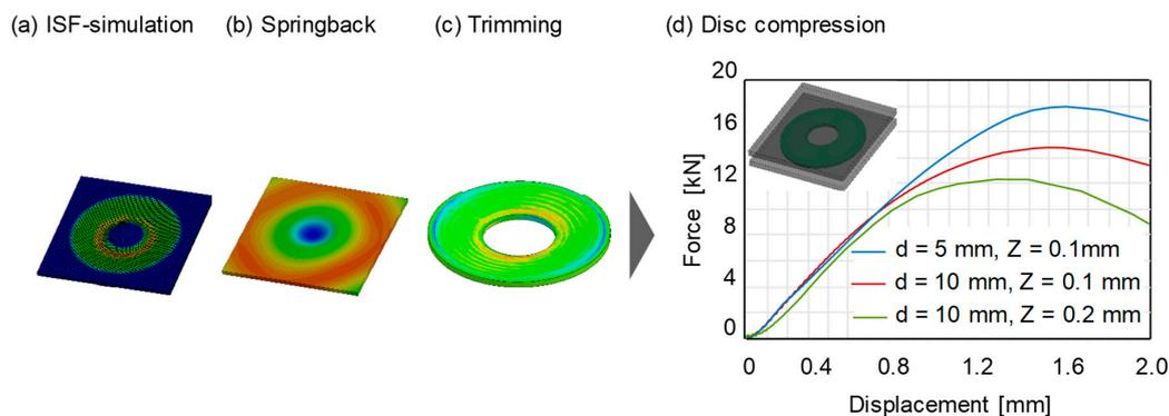
**Figure 16.** Numerical procedure for the disc compression test under varying process parameters.
