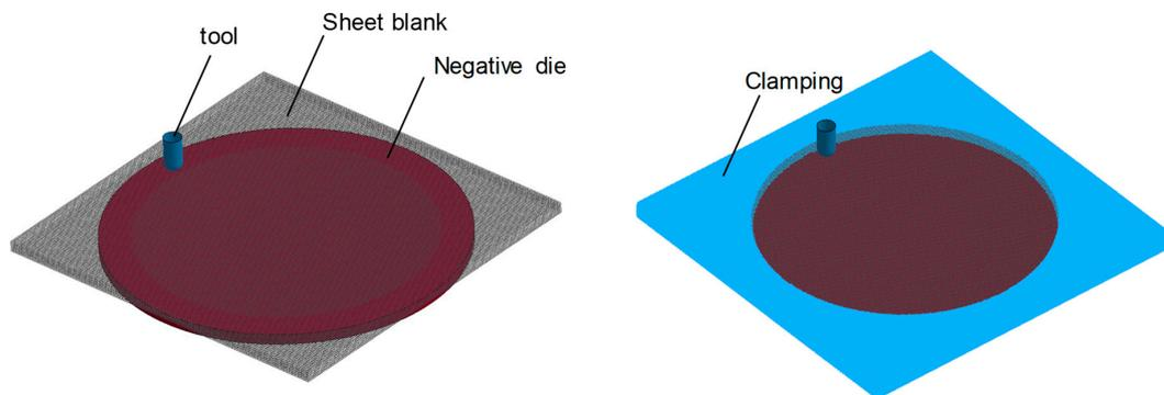
Figure 9. Model set-up for the disc spring manufacturing simulation.
