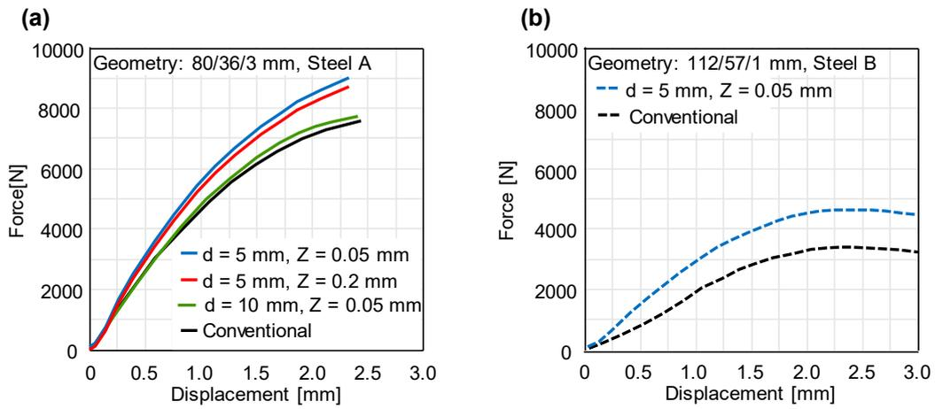
**Figure 12.** Characteristic force-displacement curves for conventional and incrementally formed disc springs from (a) steel A under varying process parameters (b) steel B.
