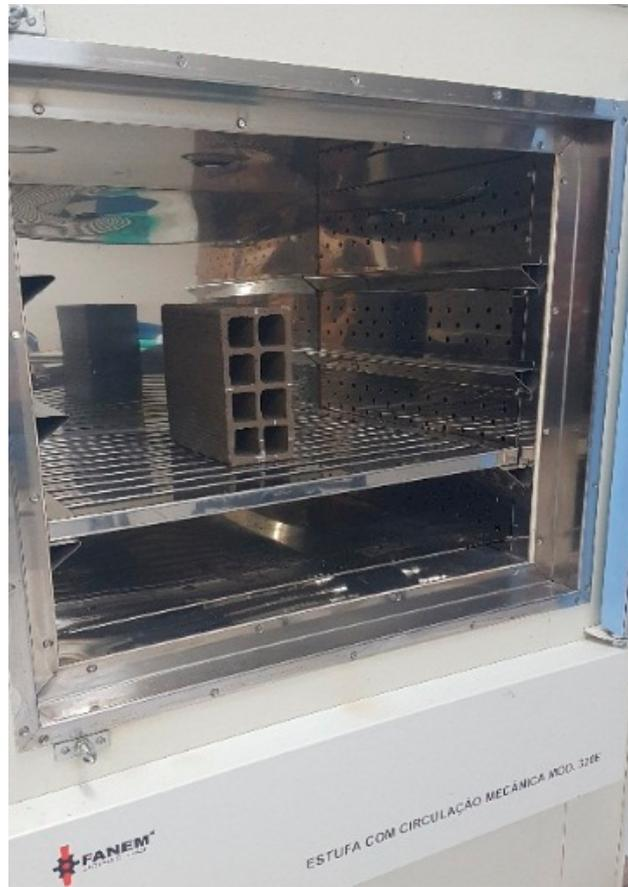
**Figure 1.** View of the ceramic brick in the drying oven (model 320E, FANEM, São Paulo, Brazil).
