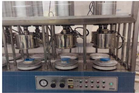
**Figure 4.** Permeability test apparatus.
