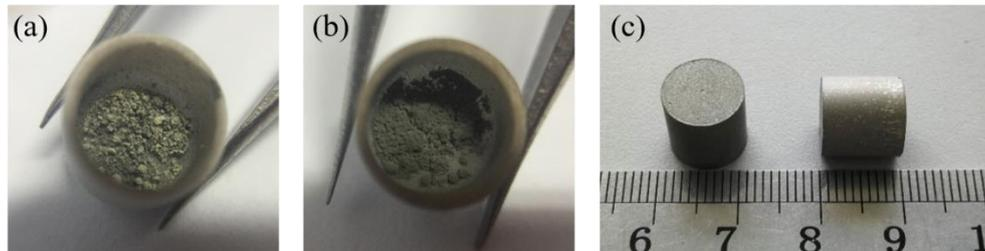
**Figure 2.** The samples used for DSC (differential scanning calorimetry) and quasi-static compression: (a) The Al-PTFE (aluminum-polytetrafluoroethene) mixture used for DSC; (b) the Al-Ni mixture used for DSC; (c) the Al-Ni-PTFE specimen used for quasi-static compression.
