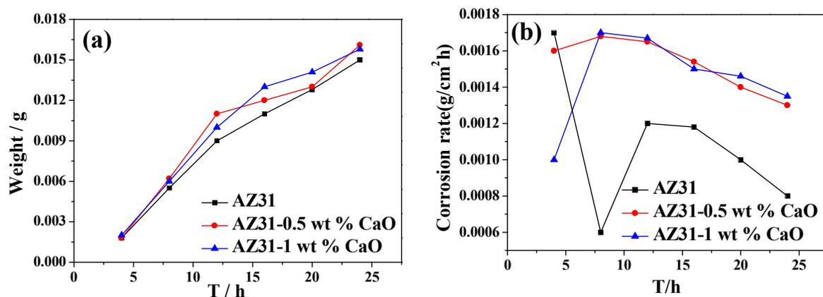
**Figure 12.** The corrosion weight loss curve (a) and corrosion rate curve (b) of AZ31-xCaO alloys.
