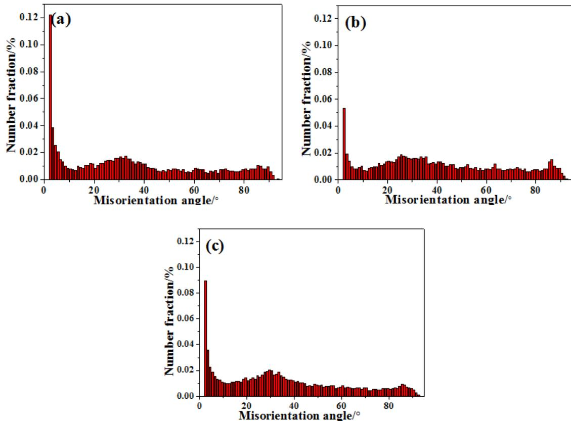
**Figure 5.** Disorientation map of grain boundary in AZ31-xCaO alloys. (a) AZ31; (b) AZ31-0.5%CaO; and, (c) AZ31-1%CaO.
