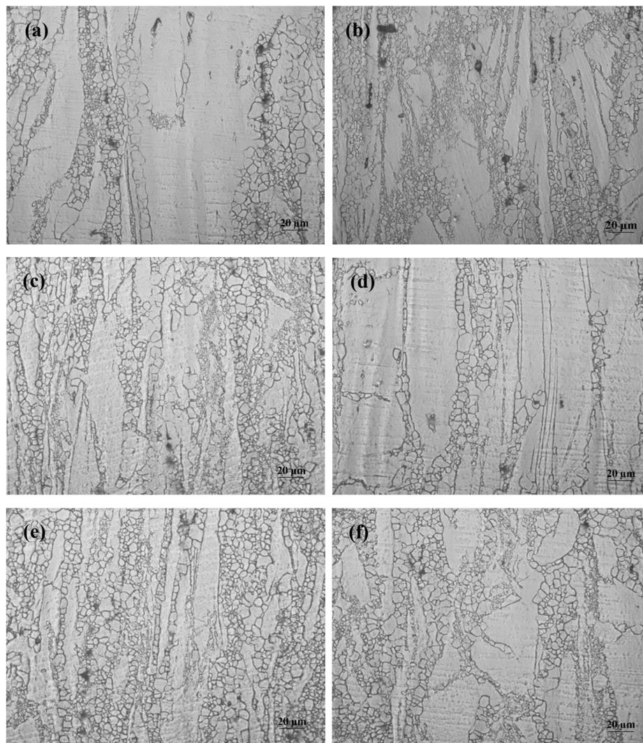
**Figure 3.** Microstructures of AZ31 (a,c,e) and AZ31-1%CaO alloy (b,d,f) at different extrusion ratios under 300 °C. (a,b) extrusion ratio is 3; (c,d) extrusion ratio is 6; and, (e,f) extrusion ratio is 9.
