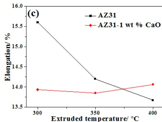
**Figure 7.** Tensile properties of AZ31 and AZ31-1%CaO alloys under different extrusion temperatures. (a) Ultimate tensile strength; (b) yield strength; and, (c) elongation.
