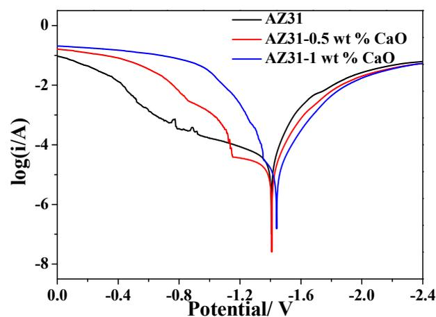
**Figure 9.** The polarization curves of AZ31-xCaO alloys.
