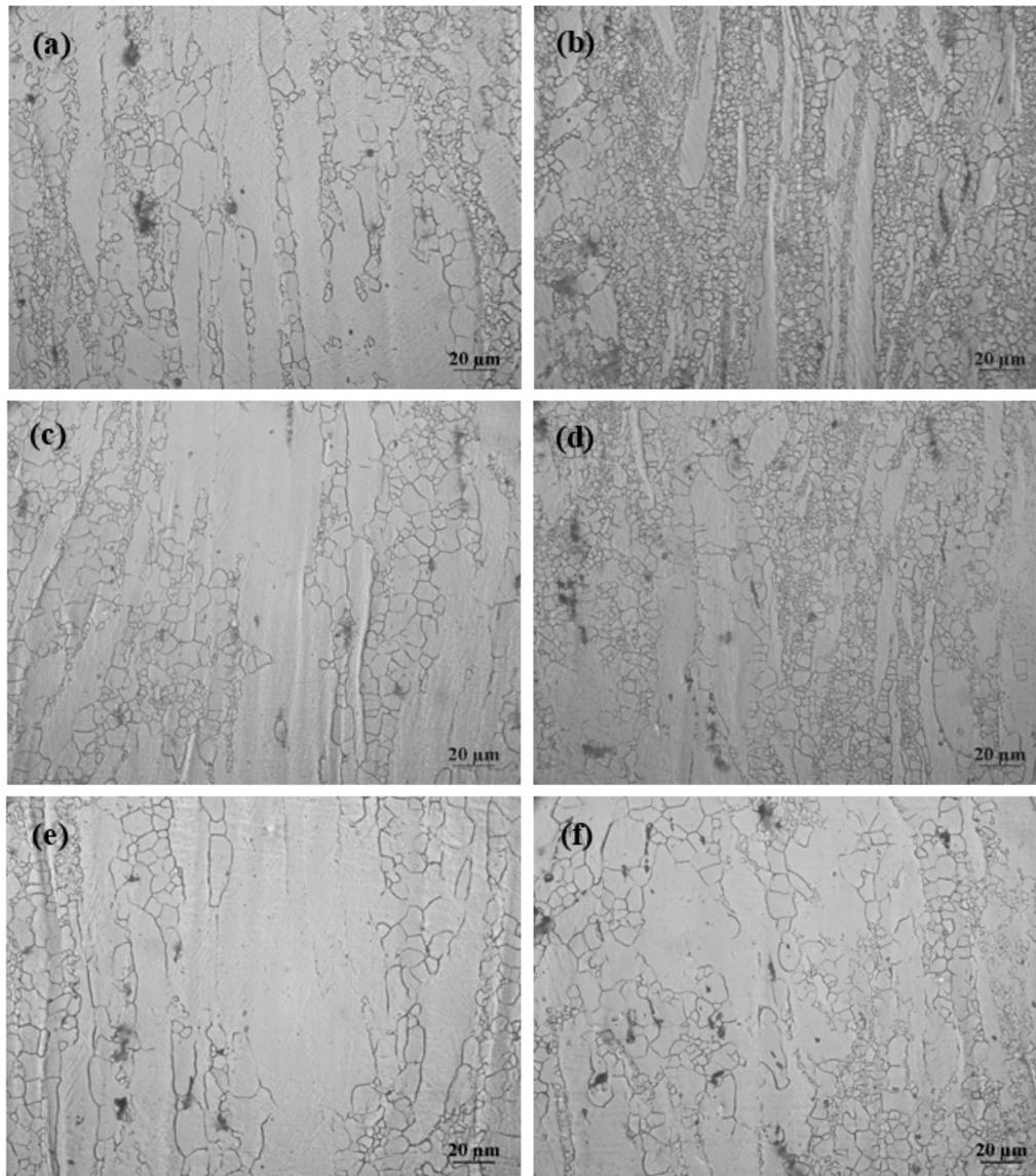
**Figure 2.** Microstructures of AZ31 alloy (a,c,e) and AZ31-1%CaO alloy (b,d,f) at a extrusion ratio of 6 under different extrusion temperatures: (a,b) 300 °C; (c,d) 350 °C; and, (e,f) 400 °C.
