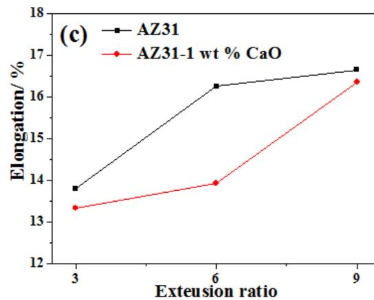
**Figure 8.** Tensile properties of AZ31 and AZ31-1%CaO alloys at different extrusion ratios. (a) Ultimate tensile strength; (b) yield strength; and, (c) elongation.
