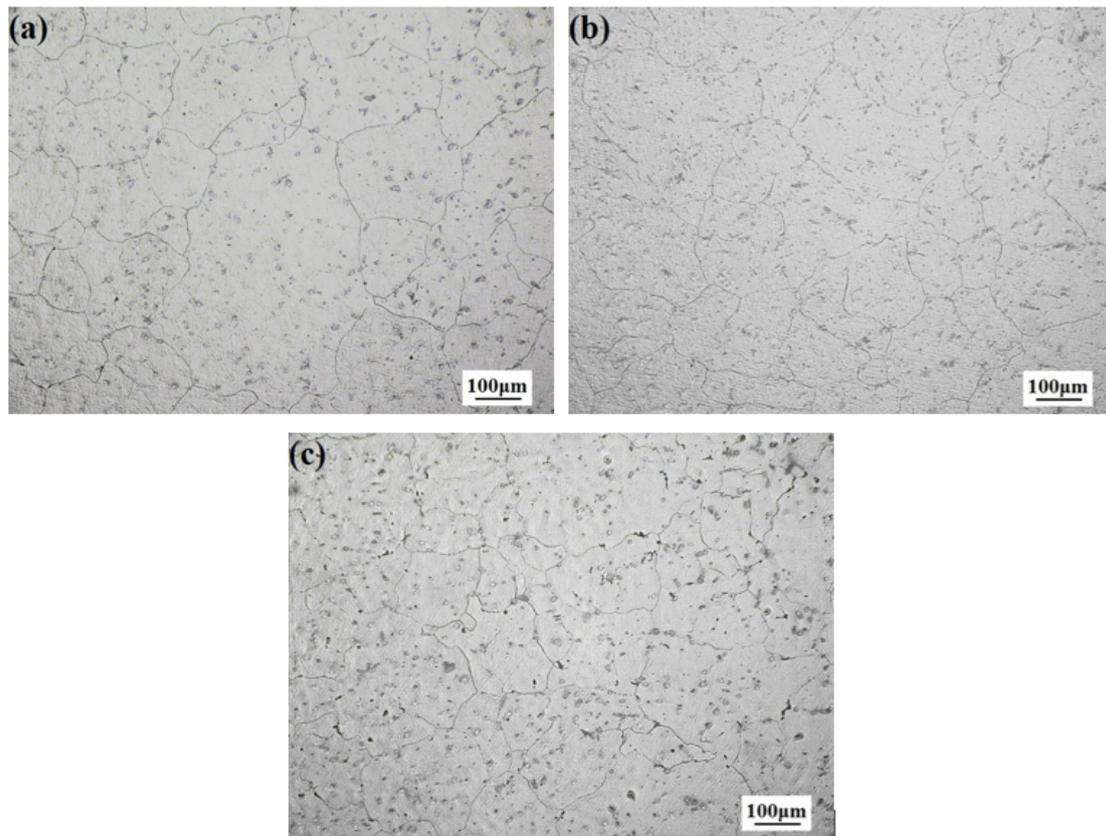
**Figure 1.** Optical microstructures of homogenization alloys. (a) AZ31; (b) AZ31-0.5%CaO; and, (c) AZ31-1%CaO.
