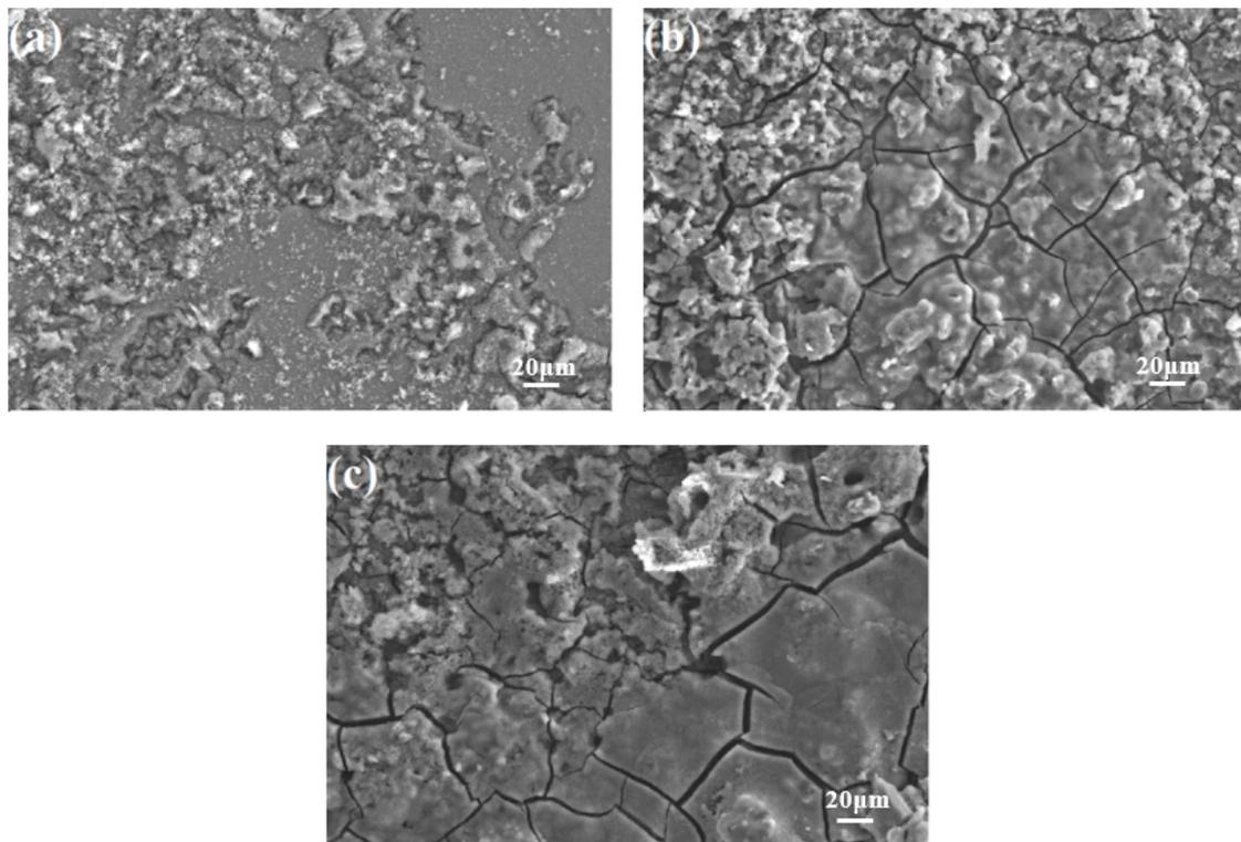
**Figure 11.** The corrosion morphologies of AZ31-xCaO alloys. (a) AZ31; (b) AZ31-0.5%CaO; and, (c) AZ31-1%CaO.
