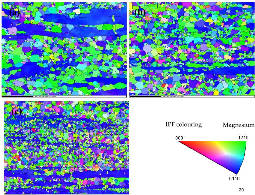
**Figure 4.** Orientation of the extruded AZ31-xCaO alloys. (a) AZ31; (b) AZ31-0.5%CaO; and, (c) AZ31-1%CaO.
