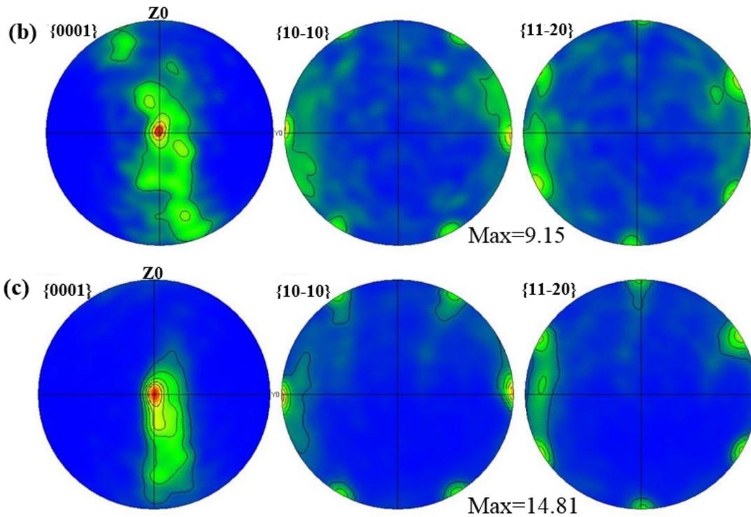
**Figure 6.** The texture strength of extruded AZ31-xCaO alloys. (a) AZ31; (b) AZ31-0.5%CaO; and, (c) AZ31-1%CaO.
