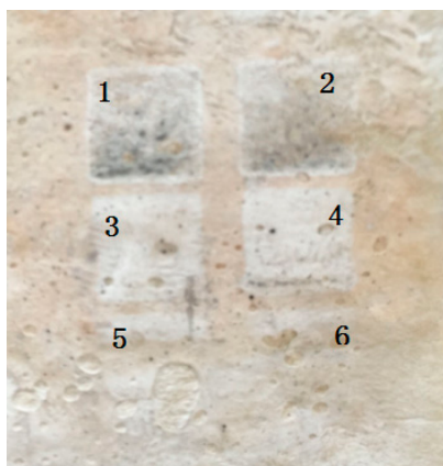
Figure 2. Effect of laser scanning speed on the Ag-deposited composite films of FP/PAN. Sample (1) 1 mm/s; (2) 2 mm/s; (3) 4 mm/s; (4) 6 mm/s; (5) 8 mm/s; (6) 10 mm/s.
