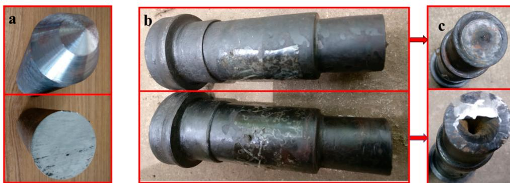
**Figure 16.** Billets and rolled products: (a) comparison of billets; (b) lateral comparison of rolled products; (c) axial comparison of rolled products.
