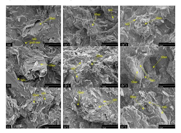
**Figure 3.** Tensile fracture surfaces of PLA hybrid composites with and without reactive compatibilizers: (a) PLA/NF2/T1; (a') PLA/NF2/T1/CEGMA; (a") PLA/NF2/T1/CEGMA/MAH; (b) PLA/NF1/T1; (b') PLA/NF1/T1/CEGMA; (b") PLA/NF1/T1/CEGMA/MAH; (c) PLA/NF1/T2; (c') PLA/NF1/T2/CEGMA; (c") PLA/NF1/T2/CEGMA/MAH.
