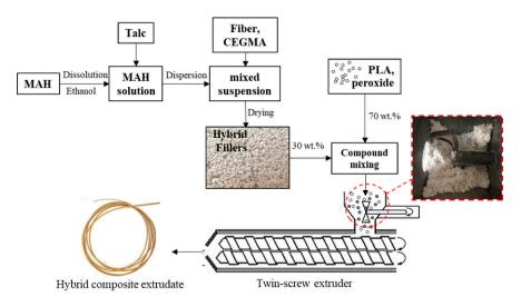
**Figure 1.** Schematic representation of the simplified preparation of hybrid fillers and extrusion compounding process of the reactive hybrid composites.
