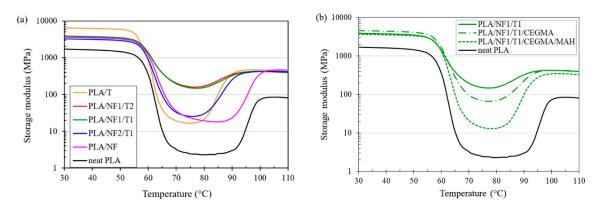
**Figure 4.** Plot of storage modulus against temperature of PLA hybrid composites at: (**a**) different fillers ratios; (**b**) with and without various reactive compatibilizers.
