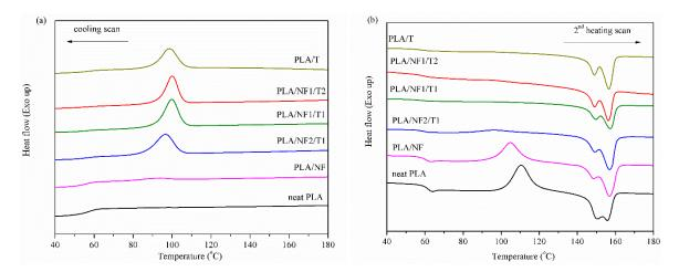
**Figure 6.** DSC thermograms of PLA hybrid composites at different filler ratios: (**a**) cooling scan and (**b**) second heating scan.
