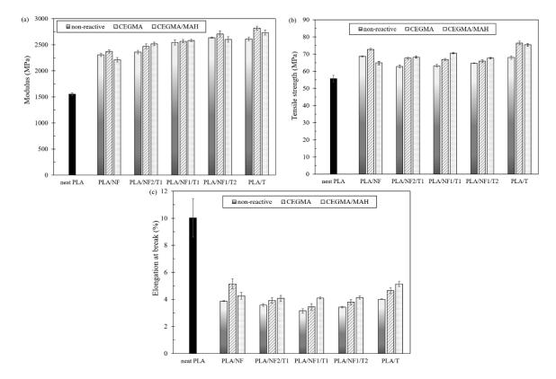
**Figure 2.** (**a**) Modulus; (**b**) tensile strength and (**c**) elongation at break of PLA hybrid composites at different fillers ratios, with and without various reactive compatibilizers.
