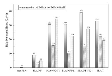
**Figure 8.** Degree of crystallinity ( $X_c$ ) of PLA hybrid composites at different filler ratios, with and without various reactive compatibilizers.
