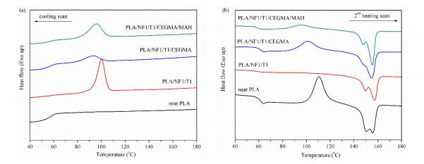
**Figure 7.** DSC thermograms of PLA hybrid composites with and without reactive compatibilizers at NF1/T1 ratio: (**a**) cooling scan and; (**b**) second heating scan.
