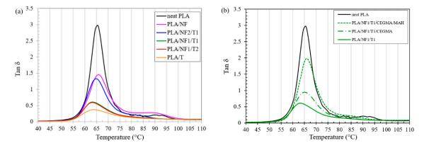
**Figure 5.** Plot of tan  $\delta$  against temperature of PLA hybrid composites at: (**a**) different fillers ratios; (**b**) with and without various reactive compatibilizers.
