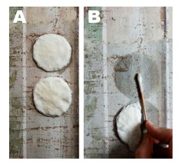
**Figure 7.** Wax removal tests performed in the Santa Croce Basilica, Florence, Italy. The wax stains appear as brownish concretions, which randomly cover the fresco surface. (**A**) Microemulsion-loaded compresses during the 2.5 h application. (**B**) Mechanical removal of the swollen and softened wax deposits by means of a humid cotton swab. Wax removal is evidenced by the brownish staining of the cotton swab tip.
