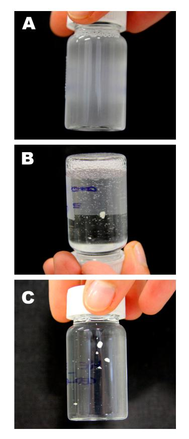
**Figure 4.** (**A**) 5 mg of paraffin emulsified in 20 mL of microemulsion; (**B**) 5 mg of beeswax swollen by 20 mL of microemulsion; (**C**) 5 mg of ceresin swollen by 20 mL of microemulsion.
