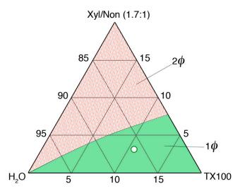
**Figure 1.** Investigated portion of the pseudo-ternary phase diagram of  $H_2O/TX100/xy$ lene:nonane (1.7:1 w/w) at 25 °C. The two-phase (red) and the single-phase (green) regions are evidenced. The white spot indicates the position of the microemulsion here reported in the phase diagram.
