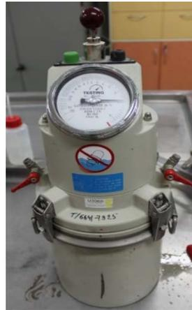
**Figure 1.** Measurement of the air content in a concrete mixture.
