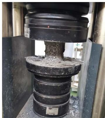
**Figure 3.** Compressive strength test of C15P1b concrete.
