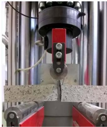
**Figure 2.** Flexural tensile strength test of C5P1b concrete.
