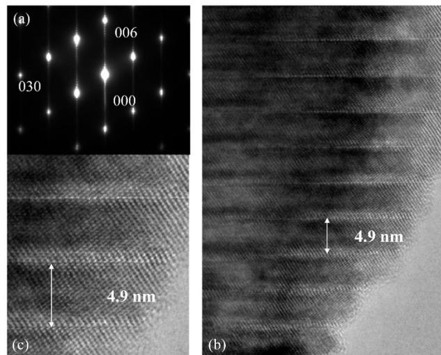
**Figure 4.** TEM images taken from the [100] axis and the selected area electron diffraction (SAED) pattern of LNT with Ti 20 mol % at 1373 K for 30 min under 0.35 MPa. (a) SAED pattern, (b) low-TEM image and (c) high-TEM image.
