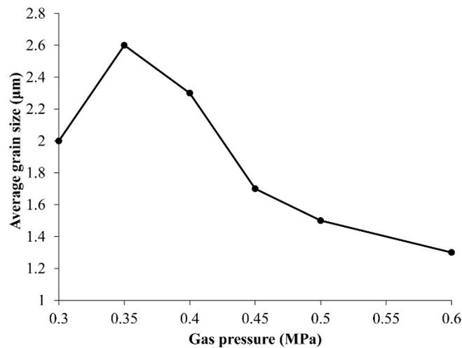
**Figure 3.** Relationship between average grain size of LNT with Ti 20 mol % and air pressure.
