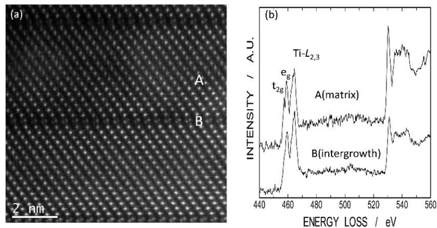
**Figure 11.** High-angle annular dark field scanning TEM (HAADF-STEM) image of LNT with Ti 20 mol % in (a) and electron energy-loss spectroscopy (EELS) data for  $L_{2,3}$ -edge of Ti ion at intergrowth layer and matrix in (b).
