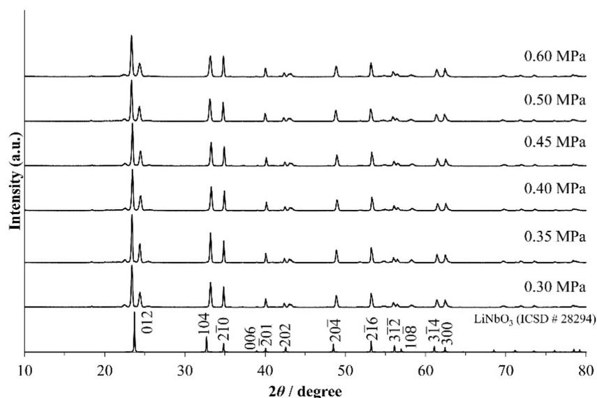
**Figure 1.** XRD patterns of  $\text{Li}_{1+x-y}\text{Nb}_{1-x-3y}\text{Ti}_{x+4y}\text{O}_3$  (LNT) solid solutions with Ti 20 mol % at 1373 K for 30 min under various air pressures.
