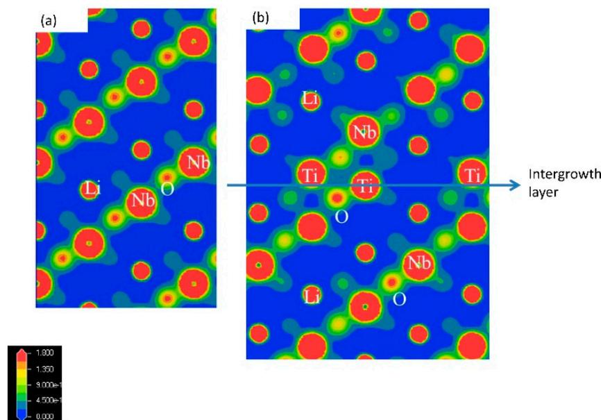
**Figure 10.** Electron density maps of  $\text{LiNbO}_3$  in (a) and  $\text{Li}_{9.5}\text{Nb}_{4.4}\text{Ti}_{7.1}\text{O}_{30}$  in (b) taken from the [100] by the first-principles molecular dynamics simulation [15].
