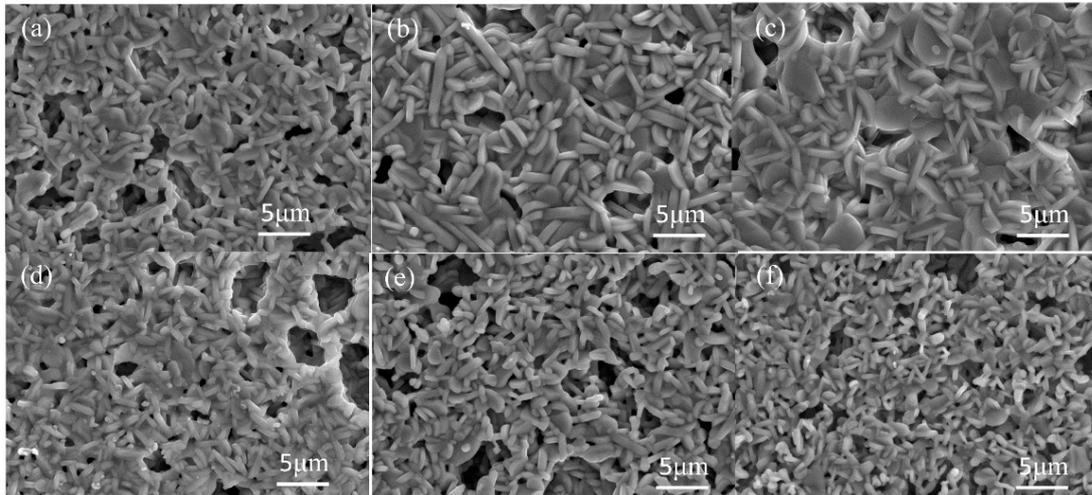
**Figure 2.** SEM images of LNT solid solutions with Ti 20 mol % at 1373 K for 30 min under various air pressures, (a) 0.30 MPa, (b) 0.35 MPa, (c) 0.40 MPa, (d) 0.45 MPa, (e) 0.50 MPa, and (f) 0.60 MPa.
