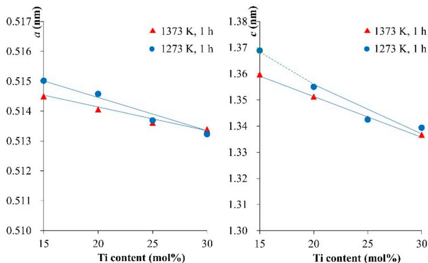
**Figure 9.** Relationship between lattice constants and Ti content.
