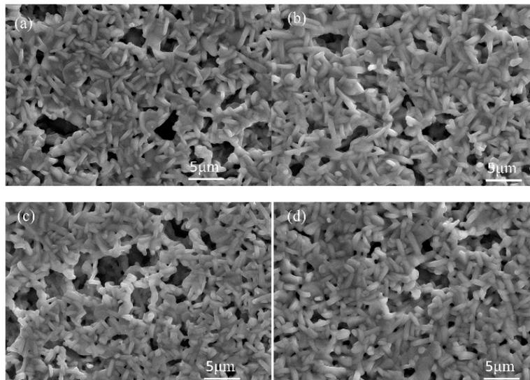
**Figure 6.** SEM images of LNT with various Ti content at 1273 K for 1 h under 0.35 MPa. (a) 15 mol %, (b) 20 mol %, (c) 25 mol %, and (d) 30 mol %.
