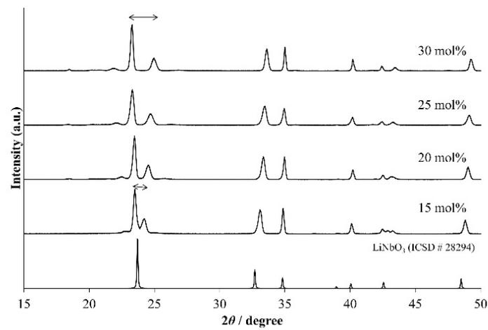
**Figure 5.** XRD patterns of LNT solid solutions with Ti 15, 20, 25, and 30 mol % at 1273 K for 1 h under 0.35 MPa.
