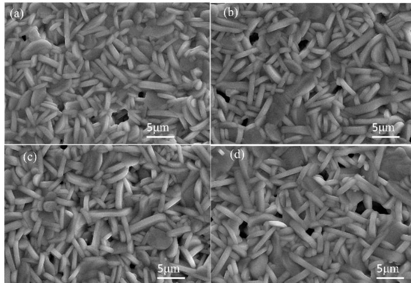
**Figure 8.** SEM images of LNT with various Ti content at 1373 K for 1 h under 0.35 MPa. (a) 15 mol %, (b) 20 mol %, (c) 25 mol %, and (d) 30 mol %.
