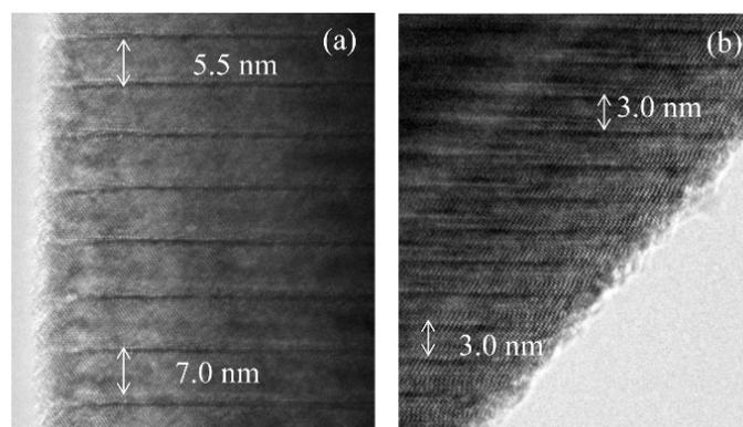
**Figure 7.** TEM images of LNT with (a) 15 mol % and (b) 30 mol % at 1237 K for 1 h under 0.35 MPa.
