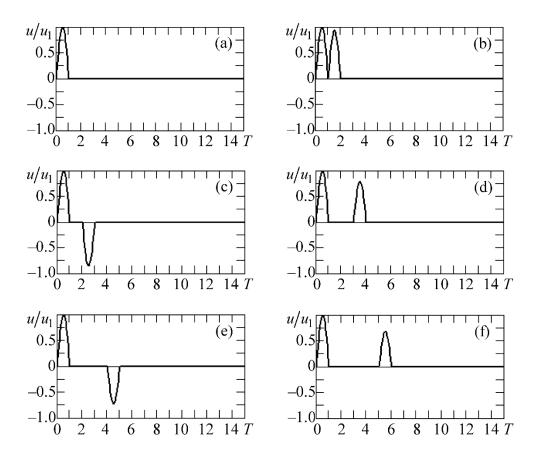
**Figure 2.** Shapes of electrical signals exciting the radiating piezoelectric plate: (**a**) shows the electric signal consisting of only one (exciting) half-period of the sine wave supplied to the radiator; (**b**–**f**) shows the electrical pulses (exciting and compensating half-waves).
