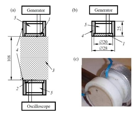
Figure 1. Experimental setup: (a) pattern, (b) diagram, and (c) photo of the piezoelectric transducer.
