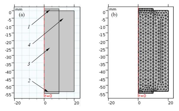
**Figure 3.** The studied geometrical area in the COMSOL Multiphysics environment: (**a**) two-dimensional (2D); (**b**) meshed simulation zone.
