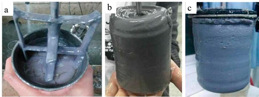
**Figure 9.** The coagulation characteristics of XNGJ-3 under different conditions: (a) under the conditions of 70 °C, 20 MPa, 2% coagulant, not consolidated; (b) under the conditions of 90 °C, 50 MPa, consolidated after 144 min; and (c) under the conditions of 120 °C, 80 MPa, 0.8% retarder, consolidated after 97 min.
