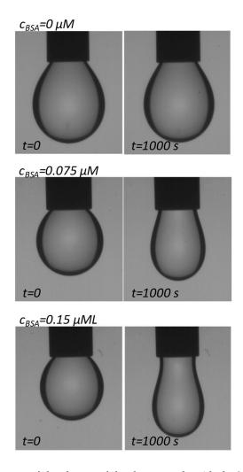
**Figure S3**. Example images of the change of the drop sample with the NPs (QD\_F NPs at 100 nM in DCM) immersed in aqueous buffer solutions at pH 5 with different BSA concentrations from the initial time (t=0) to the final measured time (t=1000 s) when the meso-equilibrium is reached. The diameter of the Hamilton needle is 1.8 mm (stainless steel NE45; Krüss-scientific).
