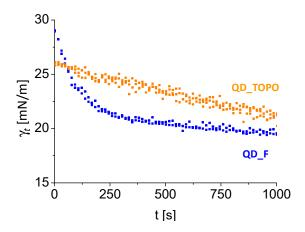
**Figure S2**. Time dependence of the interfacial tension (IFT)  $\gamma_t$  for QD\_F (100 nM in DCM) and QD\_TOPO (100 nM in DCM) immersed in aqueous buffer solution at pH 5 in the absence of proteins. Measurements were performed in triplicate.
