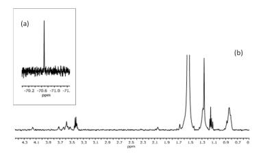
$\textbf{Figure S1.} \ (\textbf{a})^{19} F \ NMR \ spectrum \ and \ (\textbf{b}) \ ^{1}H \ NMR \ spectrum \ of \ QD\_F, \ both \ recorded \ in \ CD_{2}Cl_{2}.$
