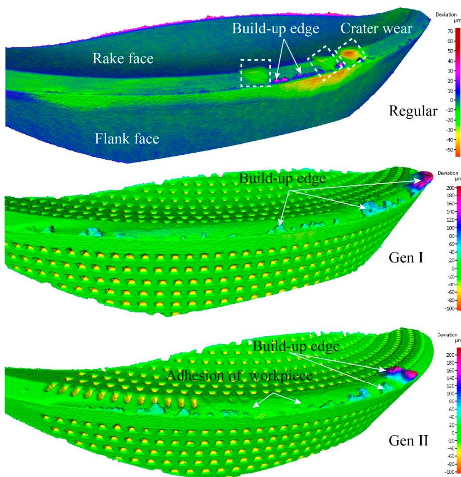
**Figure 15.** Illustration of observed different tool wear mechanism from volume difference measurement of Regular, Gen I and Gen II inserts. The topography scans are presented as the geometrical volume deviation from an unworn inserts.
