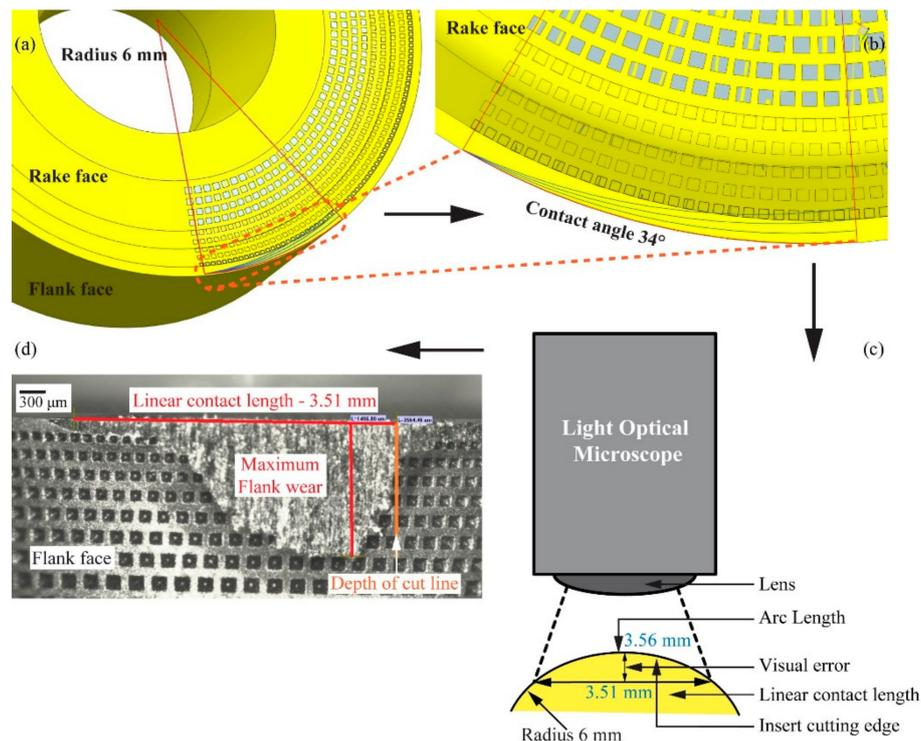
**Figure 7.** (a) Contact area of insert with  $a_p$  of 1 mm and for 6 mm insert radius; (b) magnified micrograph shows contact angle  $34^\circ$ ; (c) conversion of arc length to linear contact length; and (d) illustration of maximum flank wear measurement in relation to linear contact length of 3.6 mm and depth of cut line [9,10].
