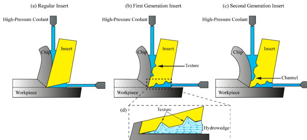
**Figure 3.** (a–c) Illustration of the interaction between the different inserts with coolant and chip, and the formation of hydro-wedges on the rake and flank face [10]; (d) magnified illustration of coolant-surface feature interaction on the flank face.
