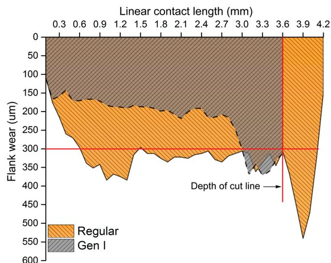
**Figure 9.** Flank wear profile of Regular and Gen I insert.
