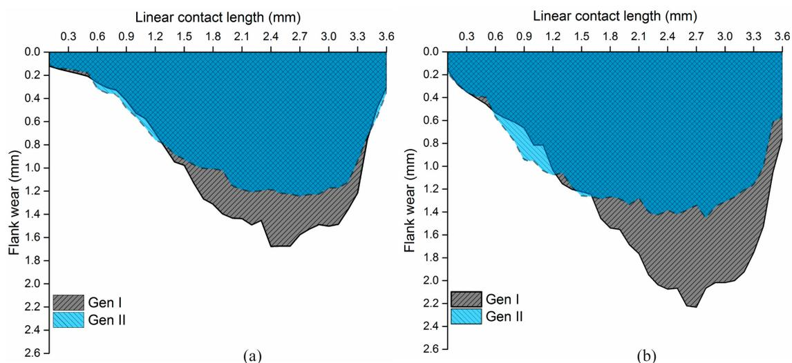
**Figure 18.** Flank wear profile of Gen I and Gen II inserts for  $f_n$  0.3 mm/rev (a)  $v_c$  90 m/min (b)  $v_c$  105 m/min.
