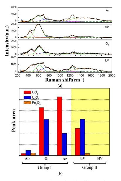
**Figure 9.** Representative Raman spectra with spectral peak fitting for center of worn surface (**a**) and the peak area (**b**).
