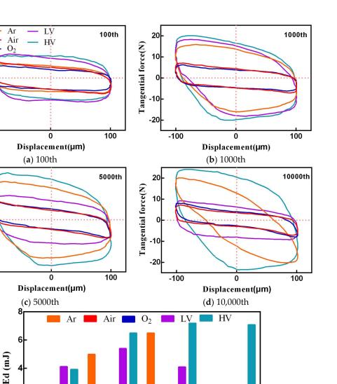
**Figure 4.** Evolution of fretting loops with cycle number under different atmosphere and vacuum conditions (**a**–**d**) and Ed of each cycles (**e**).
