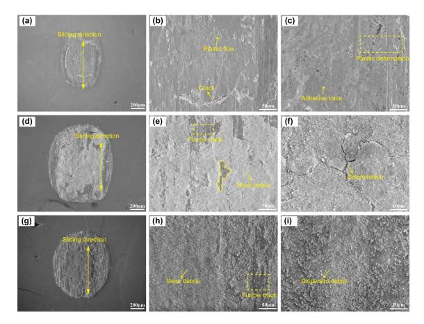
Figure 6. The SEM morphology of worn surface under Ar (a-c), Air (d-f), and O<sub>2</sub> (g-i) conditions.
