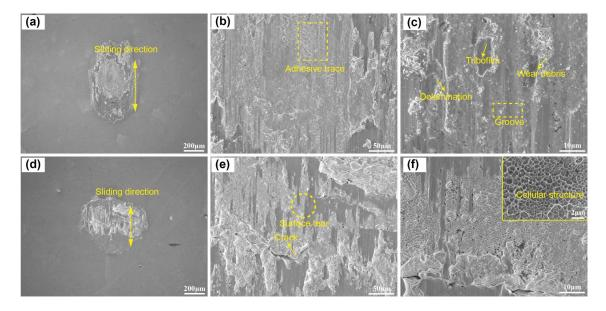
Figure 7. The SEM morphology of worn surface under LV (a–c) and HV (d–f) conditions.
