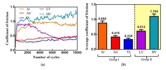
**Figure 2.** The COF versus cycle number (**a**) and the average COF under different environment conditions (**b**).
