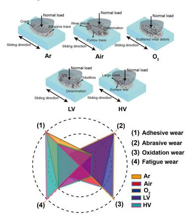
**Figure 11.** Schematic diagrams of the wear model and wear mechanism of uranium under different atmosphere and vacuum conditions.
