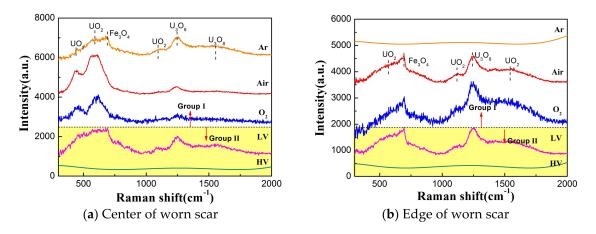
Figure 8. The Raman spectrum of the wear surface under different atmosphere and vacuum conditions.
