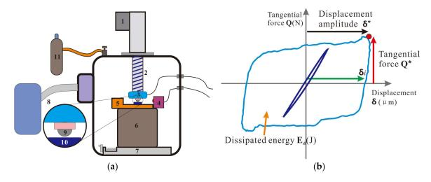
**Figure 1.** Schematic view of experimental equipment (**a**) and fretting loop analysis (**b**). (**1**) servo electric cylinder; (**2**) lead screw; (**3**) three-dimensional pressure sensor; (**4**) laser copolymerization sensor; (**5**) piezoelectric ceramics; (**6**) base; (**7**) screw module; (**8**) vacuum pump system; (**9**) ball sample; (**10**) plate sample; (**11**) gas transmission system.
