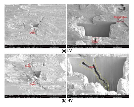
Figure 10. Cross-section images of the worn surface under different vacuum conditions. (a) LV; (b) HV.
