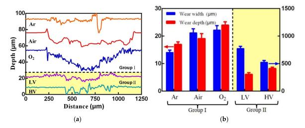
**Figure 3.** The profile micrographs of wear scars (**a**) and the corresponding wear width and wear depth (**b**) under different atmosphere and vacuum conditions.
