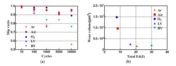
**Figure 5.** Evolution of slip ratio with cycle number (**a**) and Ed versus wear volume under different atmosphere and vacuum conditions (**b**).
