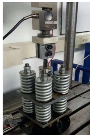
Figure 2. Specimen mounted on the uniaxial fatigue machine.
