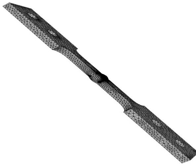
Figure 4. Detail of the mesh generation for the weld joint model.
