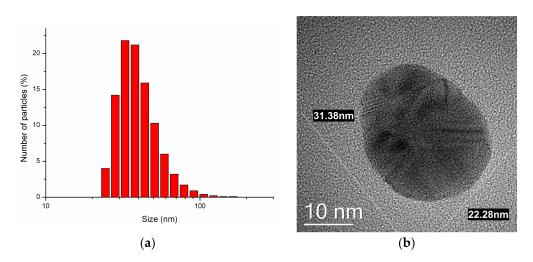
**Figure 1.** (a) Distribution of a number of particles by size for the initial measurements with Argovit C delivered with Dynamical Light Scattering (DLS); (b) Microphotograph of Argovit C silver nanoparticle Ag-NP visualized by Transmission Electron Microscopy (TEM).
