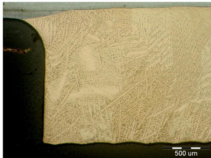
**Figure 8.** Dendritic microstructure of CuSn6P cladding.
