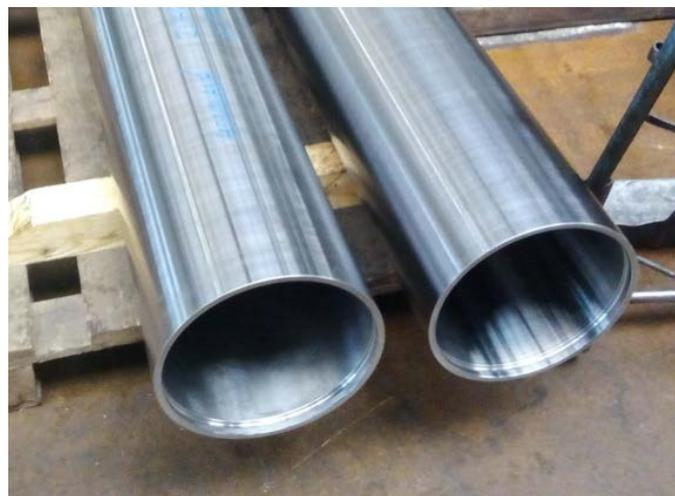
**Figure 3.** Workpiece steel cylinders before the application of bronze cladding.
