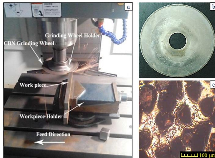
**Figure 2.** The detailed information of experiment setup: (a) The experiment setup; (b) the electroplated monolayer CBN; (c) CBN abrasive distribution.
