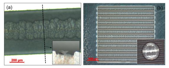
**Figure 3.** (a) Top view of the re-entrant structure realized by building the additive structures (AS) block from two sides. The dash line and the arrow are the visual indication of a cross-section. The inset is a cross-section of this re-entrant structure; (b) The structure unit shown in (a) is easily implemented on a large surface scale. This surface exhibits isotropic hydrophobicity (lower bottom inset).
