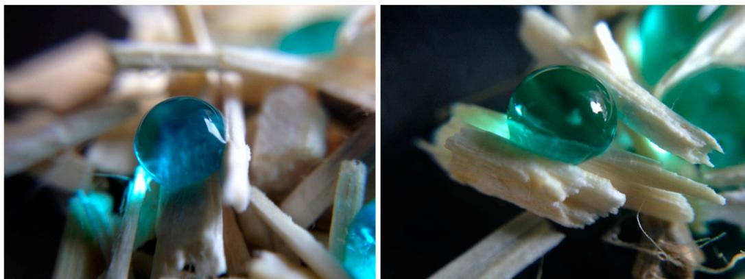
**Figure 8.** Coloured water droplets onto hemp shiv H12-1-5, with a WCA > 125°. Courtesy of TWI Ltd.
