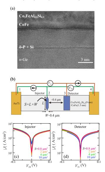
**Figure 2.** (a) Cross-sectional TEM image of the FM/*n*-Ge interface of a measured lateral spin valve (LSV) device; (b) Schematic illustration of the terminal configuration for |J|-V measurements; |J|-V curves for (c) spin injector and (d) spin detector with various contact sizes at 30 K.
