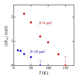
**Figure 5.** Temperature dependence of spin signal for LSVs with S = 4 (circle) and 10 (diamond)  $\mu$ m<sup>2</sup>.
