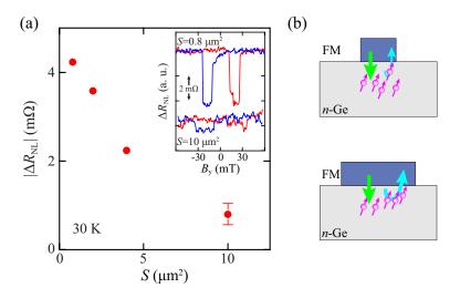
**Figure 4.** (a) *S* dependence of  $|\Delta R_{\text{NL}}|$  at 30 K. The inset shows the nonlocal spin signal for the LSVs with *S* = 0.8 and 10  $\mu$ m<sup>2</sup>; (b) Schematic diagram of spin absorption effect under the small and large FM contacts.
