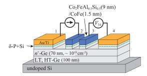
**Figure 1.** Schematic illustration of the fabricated lateral spin valve with ferromagnet (FM)/Ge Schottky-tunnel contacts. HT: high-temperature-grown; LT: low-temperature-grown.
