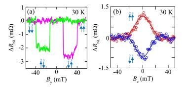
**Figure 3.** Four-terminal nonlocal (**a**) magnetoresistance curve and (**b**) Hanle-effect curves for the parallel and antiparallel magnetization configurations at 30 K. The solid curves in (**b**) indicate the results fitted to Equation (2) in Ref. [37].
