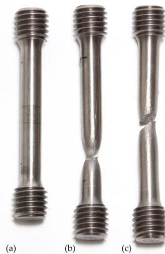
**Figure 7.** Exemplary depiction and visual comparison of the tensile test specimens according to ISO 6892-1 before (a) and after (b,c) tensile tests. Seven of the eight fractured specimens markedly displayed the typical necking (b), whereas one of the specimens (c) showed shear fracture.
