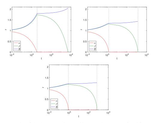
**Figure 4.** Plots of the dimensionless variables  $\alpha$ ,  $\beta$  and S against t, from left to right, Cartesian, cylindrical and spherical geometry using  $\varepsilon_1 = 0.6$ ,  $\varepsilon_2 = 0.4$ ,  $\kappa \to \infty$ , the parameters in Table 4 and  $S_0 = 1$ . The dashed lines show  $t = T_{\alpha}$  (left) and  $T_{\beta}$  (right).
