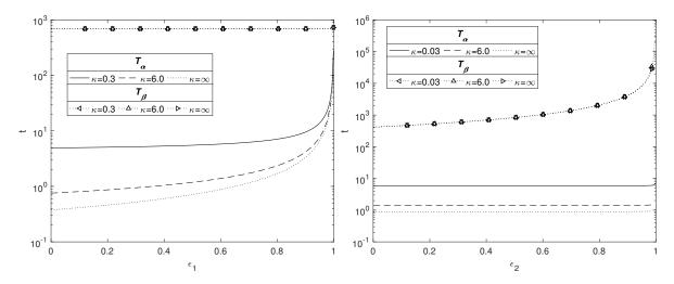
**Figure 6.** Plots of the dimensionsionless  $T_{\alpha}$  and  $T_{\beta}$  against  $\varepsilon_1$  (**left**) and  $\varepsilon_2$  (**right**) for  $\kappa = 0.03, 6$  and  $\kappa \to \infty$ , with the remaining parameters listed in Table 4 and  $S_0 = 1$ .
