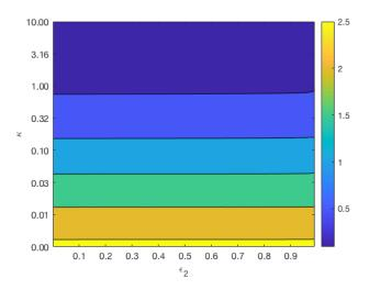
**Figure 7.** Contour map of the dimensionless  $T_{\alpha}$  for  $\kappa$  against  $\varepsilon_1$  with  $\varepsilon_2 = 0.4$  (**top**) and  $\kappa$  against  $\varepsilon_2$  with  $\varepsilon_1 = 0.6$  (**bottom**) in spherical geometry. The remaining parameters are listed in Table 4 and  $S_0 = 1$ .
