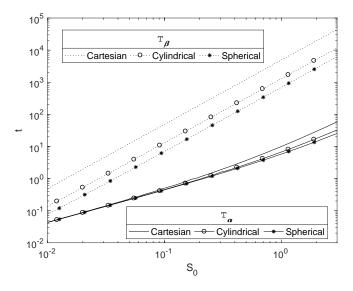
**Figure 5.** Plots of the dimensionsionless  $T_{\alpha}$  and  $T_{\beta}$  against the initial magnesium block size,  $S_0$ , for each of the principle geometries. The parameters used are  $\varepsilon_1 = 0.6$ ,  $\varepsilon_2 = 0.4$ ,  $\kappa \approx 0.3$  ( $k = 0.5 \text{ cm}^4/\text{g day}$ ) and parameters in Table 4.
