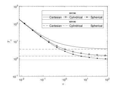
**Figure 8.** Plots of the dimensionsionless  $T_{\alpha}$  against  $\kappa$  for the three principle geometries, with  $\varepsilon_1 = 0.6$   $\varepsilon_2 = 0.4$ ,  $S_0 = 1$  and the parameters listed in Table 4.
