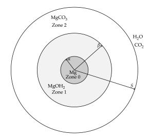
**Figure 1.** A physiochemical schematic of the magnesium corrosion system used in the model for cylindrical and spherical geometries. The pure magnesium or magnesium alloy exists in the core (Zone 0,  $0 \le r < \alpha(t)$ ), the magnesium hydroxide forms a middle layer (Zone 1,  $\alpha(t) < r < \beta(t)$ ) and the outer layer consists of magnesium carbonate (Zone 2,  $\beta(t) < r < S(t)$ ).
