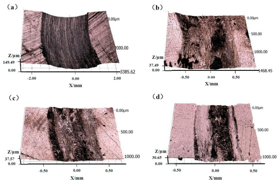
Figure 9. 3D non-contact surface mapping of the wear scars of (a) substrate; (b) 0Mo coating; (c) 4Mo coating and (d) 8Mo coating.
