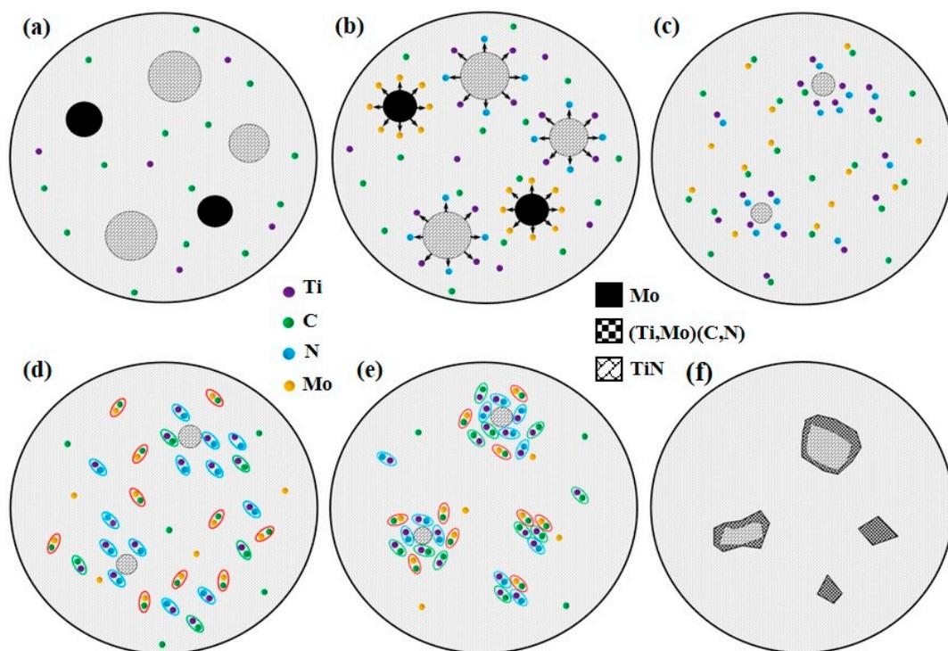
**Figure 5.** The diagram illustration for the formation mechanism of Ti(C,N) and the action mechanism of Mo: (a) the formation of initial molten pool; (b) dissolution of TiN and Mo; (c) partially melted large TiN particles; (d) the formation of TiN, TiC and MoC; (e) the formation and growth of Ti(C,N); (f) the effect of Mo on the Ti(C,N).
