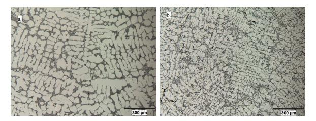
Figure 2. Optical microstructures of the (a) initial alloy and (b) alloy treated by oxygen blowing.
