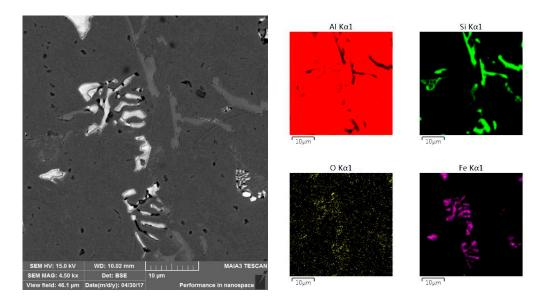
**Figure 4.** Scanning electron microscopy image of the  $Al_{10}$ SiFe complex intermetallic compound and energy dispersive spectroscopy (EDS) mapping analysis of the image.
