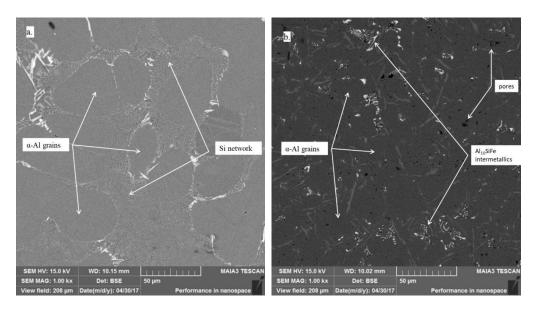
**Figure 3.** Scanning electron microscopy images of (**a**) the initial alloy and (**b**) the alloy treated by oxygen blowing.
