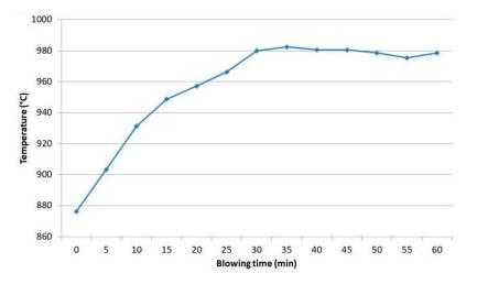
**Figure 1.** AlSi<sub>7</sub>Fe<sub>1</sub> casting alloy temperature mode as a function of oxygen blowing.
