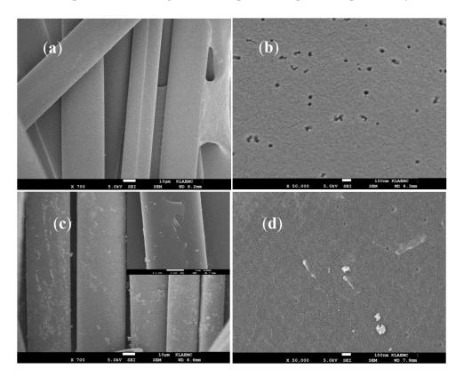
**Figure 1.** Scanning electron micrographies of the surface of wood-based activated carbon fiber (WACF) (**a**,**b**) and Mn/TiO<sub>2</sub>–WACF (**c**,**d**).
