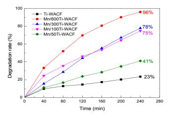
**Figure 7.** Degradation curve chart of methylene blue by samples with different Mn-doping concentrations under visible lights.
