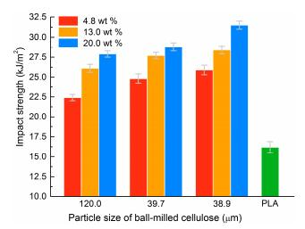
**Figure 4.** Impact strength of the cellulose/PLA composite materials. The green bar means the impact strength of pristine PLA, which is used as reference.
