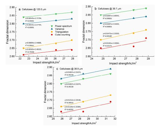
**Figure 5.** Correlation between fractal dimension and impact strength of the PLA-based composite materials reinforced with ball-milled celluloses. The particle size of ball-milled cellulose shown in (a-c) of Figure 5 is 120.0, 39.7, and 38.9 µm, respectively.
