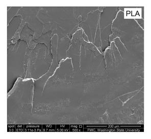
Figure 2. SEM images of the fracture surfaces of PLA.
