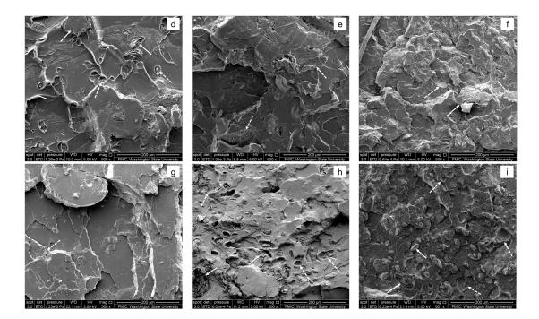
**Figure 3.** SEM images of the impact fractured surfaces of cellulose/PLA composite materials. The letters **a**–**i** are used to show their different composition for the composite materials (see the details in Table 1). The arrows mean the ball-milled cellulose particles filled in PLA. The dotted arrows mean the traces left by the cellulose particles pulled out from the matrix.
