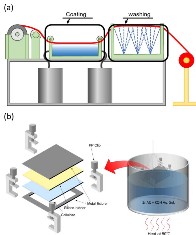
**Figure 1.** Concepts of (a) a continuous production of a hydrothermally synthesized ZnO nanocoating on a cellulose film (HZONCE) and (b) laboratory-scale fabrication setup.
