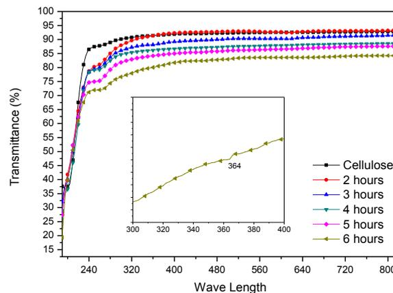
**Figure 4.** Transparency of the initial HZONCEs depending on the reaction time.
