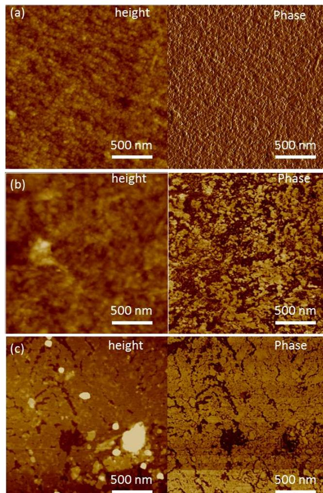
**Figure 7.** AFM images in terms of height and phase for the improved HZONCEs depending on the reaction time: (a) cellulose; (b) twice-1 h; (c) twice-3 h.
