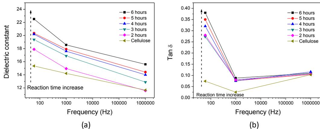
**Figure 5.** (a) Dielectric constant and (b) dielectric  $\tan \delta$  of the initial HZONCEs depending on the reaction time.
