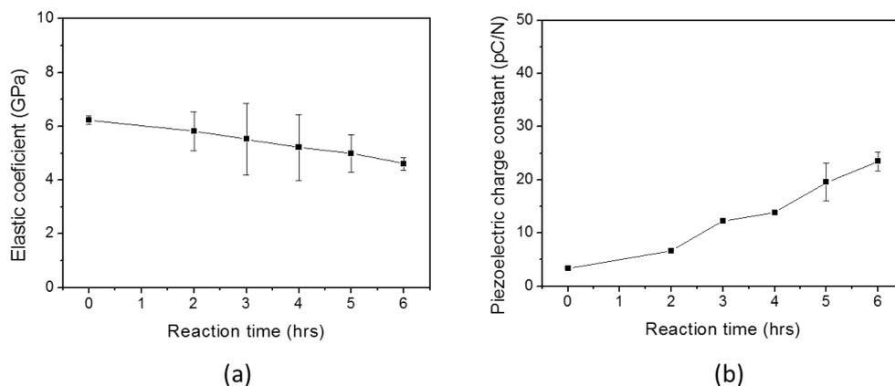
**Figure 6.** (a) Young's modulus and (b) piezoelectric charge constant of the initial HZONCEs depending on the reaction time.
