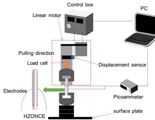
**Figure 2.** Experimental setup for pull test.
