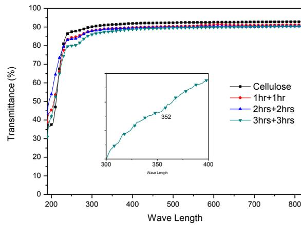
Figure 9. Transparency of the improved HZONCEs depending on the reaction time.
