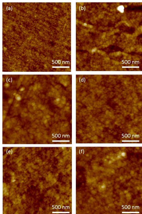
**Figure 3.** Atomic force microscopy (AFM) images of the initial HZONCEs depending on the reaction time: (a) cellulose; (b) 2 h; (c) 3 h; (d) 4 h; (e) 5 h; and (f) 6 h.
