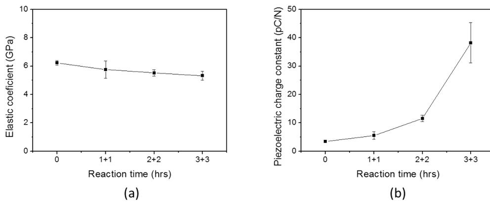
Figure 11. (a) Young's modulus and (b) piezoelectric charge constant of twice HZONCEs depending on reaction time.
