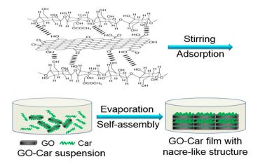
Figure 1. Scheme for fabricating green graphene oxide-carrageenan (GO-Car) composite films.
