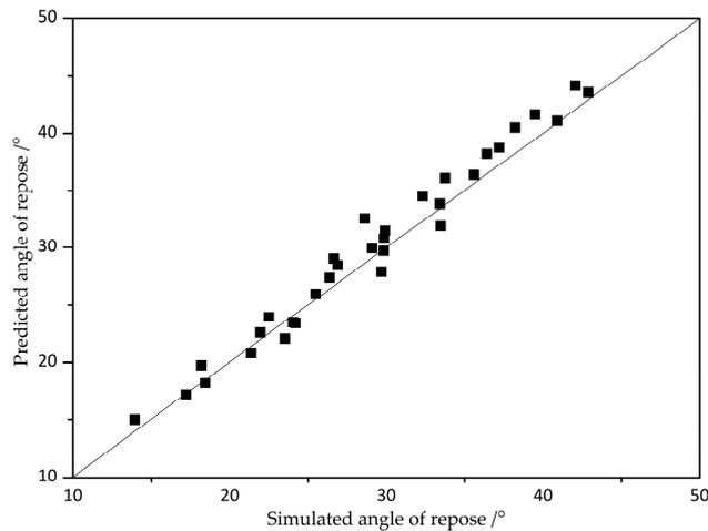
**Figure 11.** The effect of the simulated angle of repose with the predicted angle of repose.
