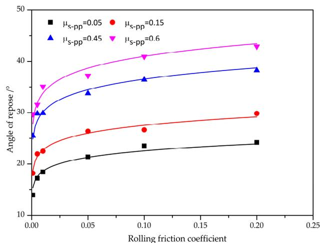
**Figure 10.** The effect of the rolling friction coefficient on the angle of repose.
