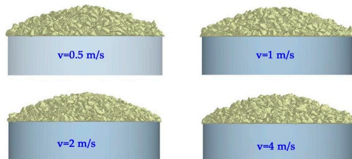
**Figure 7.** Effect of velocity on angle of speed when  $e_{pp} = 0.05$ ,  $\mu_{s-pp} = 0.15$ ,  $\mu_{r-pp} = 0.01$ .
