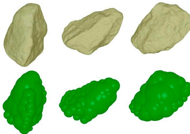
Figure 2. Iron ore particle modelling by the sphere clump method (60 spheres).
