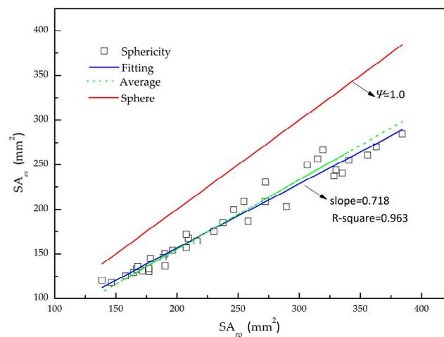
Figure 4. Sphericity of thirty-six iron ore particles.
