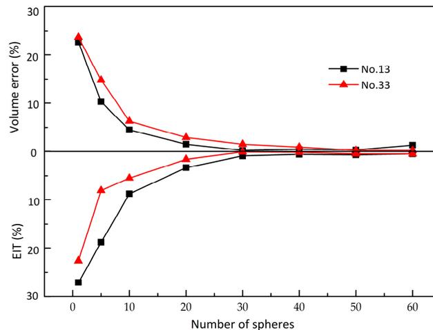
**Figure 6.** The change in volume error and EIT error with number of sphere clumps.
