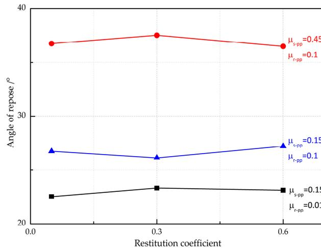
Figure 8. Effect of the restitution coefficient on the angle of repose.
