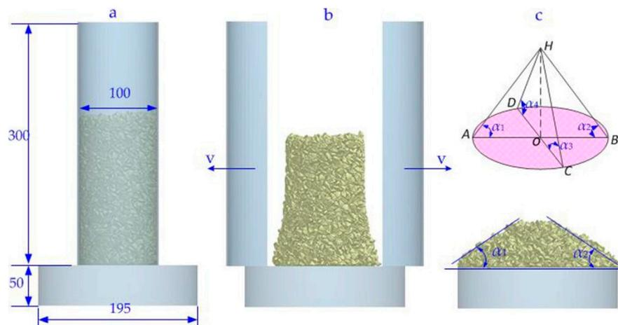
**Figure 3.** Forming process of the particle pile on the plane. (a) Initial state of the simulation; (b) being in the particle's accumulating; (c) sand-pile stabilized.
