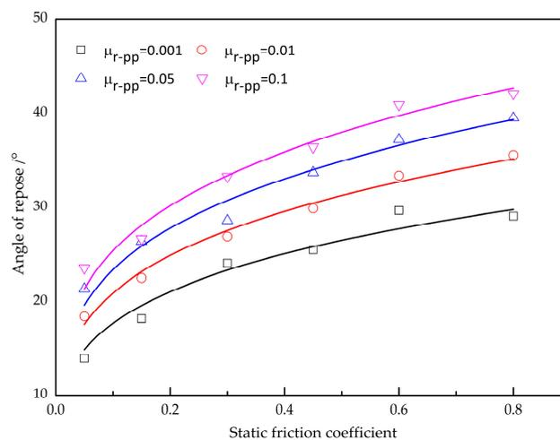
Figure 9. The effect of the static friction coefficient on the angle of repose.
