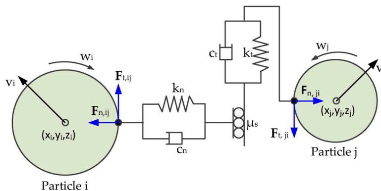
Figure 1. The illustration of the contact forces between particle  $i$  and particle  $j$ .
