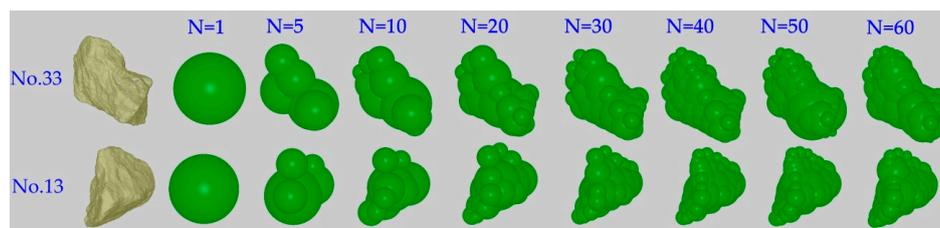
Figure 5. The geometrical model of iron ore particles with various numbers of sphere clumps.
