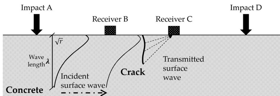
Figure 3. Transmission of surface waves across a crack.
