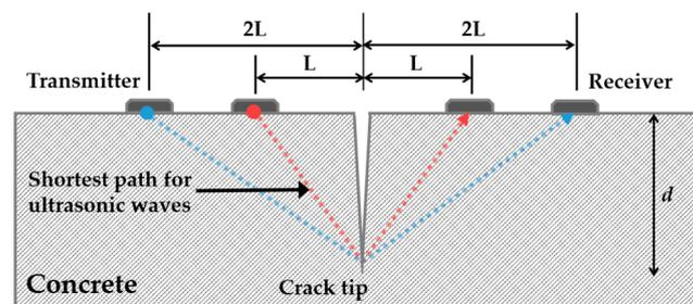
**Figure 7.** Concepts of time-of-flight diffraction (TOFD) methods.
