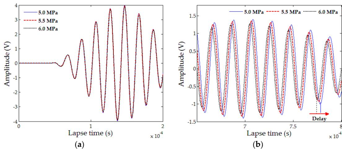
**Figure 5.** Typical ultrasonic wave signals in concrete: (a) earlier parts and (b) later parts [58].
