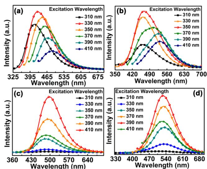
Figure 2. PL spectra of (a) CDs-COOH, (b) S1, (c) S2, and (d) S3 excited with different wavelengths.
