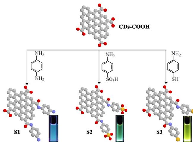
**Figure 1.** Schematic of modifying CDs with p-phenylenediamine (S1), sulfanilic acid (S2), and 4-aminothiophenol (S3), respectively, and their corresponding emission photos under UV excitation of 356 nm.
