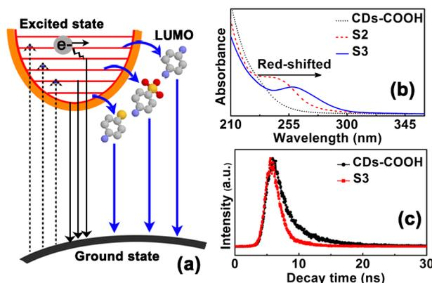
**Figure 5.** (a) Illustration for the PL mechanism of modified CDs; (b) Light absorption comparisons of CDs-COOH, S2, and S3; (c) PL decay profiles of CDs-COOH and S3 excited by the same wavelength.
