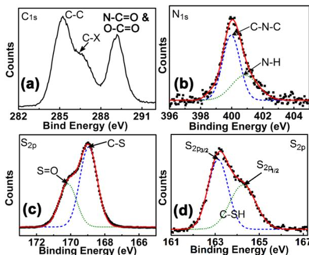
**Figure 4.** XPS spectra for modified CDs (a) a typical C<sub>1s</sub>; (b) N<sub>1s</sub>; (c) S<sub>2p</sub> of S<sub>2</sub> and (d) S<sub>2p</sub> of S<sub>3</sub>.
