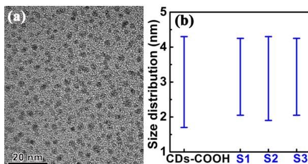
**Figure 3.** A typical TEM image of (a) CDs and (b) the size distributions of CDs-COOH, S1, S2, and S3.
