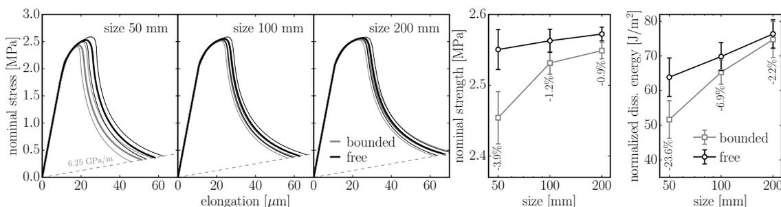
**Figure 12.** left: comparison of the averaged responses of a periodic 3D model of concrete with  $\alpha = 0.29$  loaded in pure tension; right: comparison of strength and dissipated energy.
