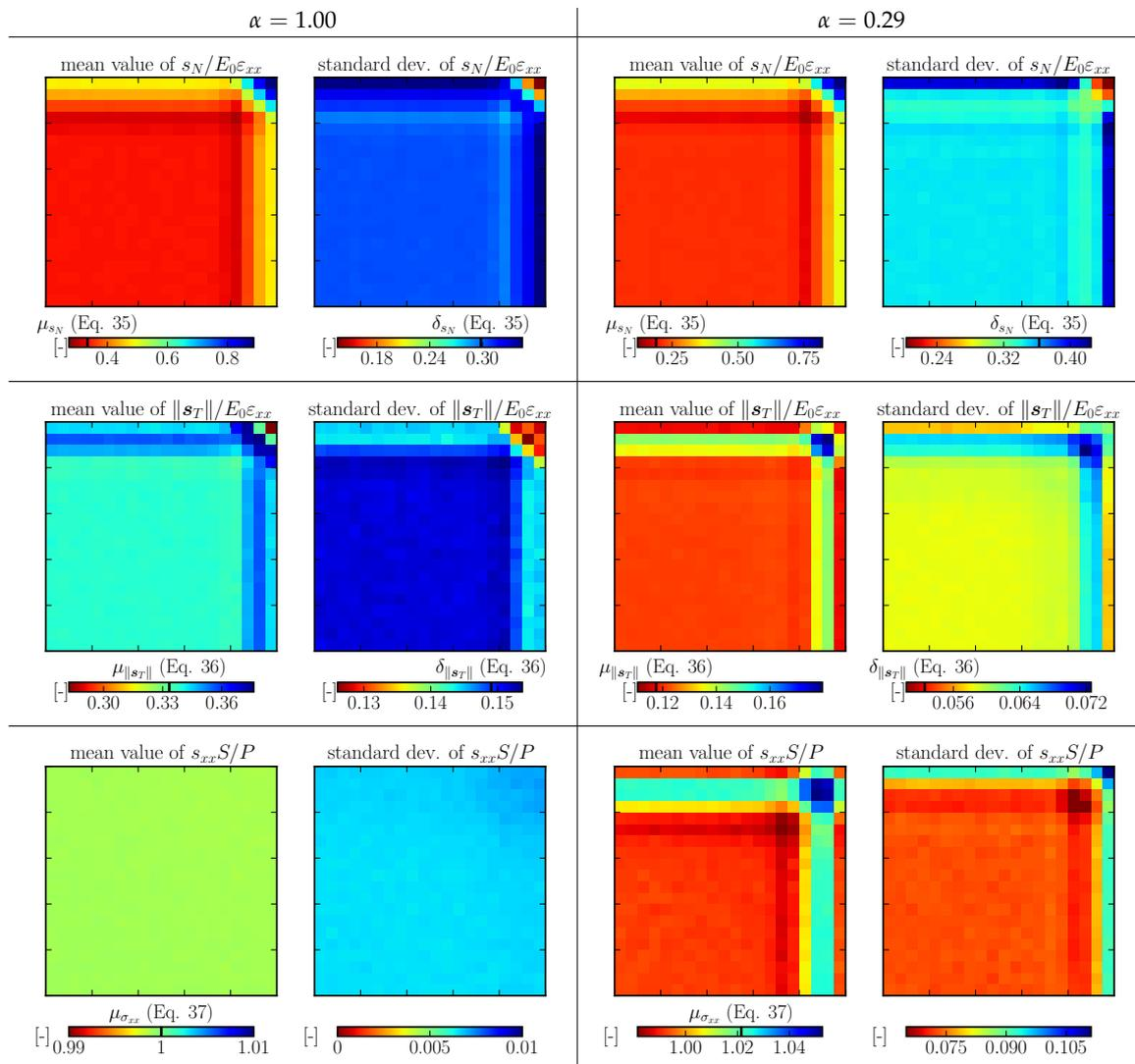
Figure 9. Average and standard deviation of normal stress, shear stress and tensorial stress; 3D model.
