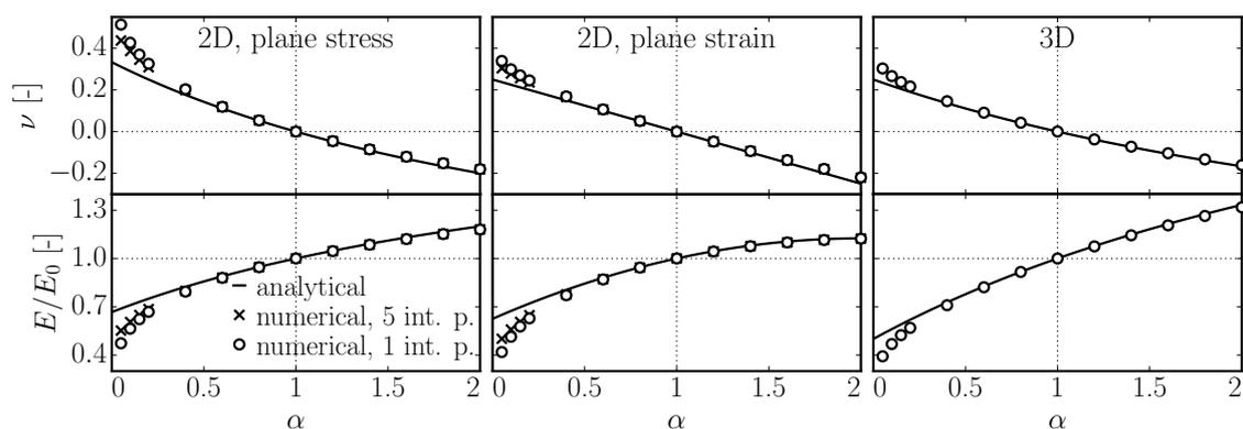
**Figure 5.** Comparison of macroscopic elastic modulus and Poisson's ratio estimated analytically (Equation (25)) and computed numerically on a large discrete system.
