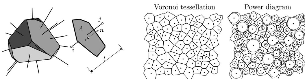
**Figure 1.** left: one rigid body and one contact facet connecting nodes  $i$  and  $j$  with normal  $\mathbf{n}$ , length  $l$  and area  $A$ ; right: Voronoi tessellation and Power diagram for the same set of nuclei.
