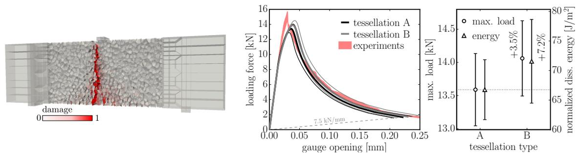
Figure 13. left: beam loaded in three-point bending; right: results averaged over 100 simulations.
