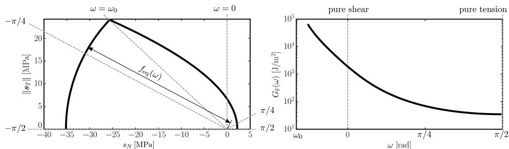
**Figure 3.** Constitutive relations for material parameters used in nonlinear models ( $E_0 = 60$  GPa,  $\alpha = 0.29$ ,  $f_t = 2.2$  MPa and  $G_t = 35$  J/m<sup>2</sup>); length of the element is  $l = 10$  mm. left: elastic envelope  $f_{eq}$  for different  $\omega$ ; right: fracture energy  $G_F$  dependent on straining direction  $\omega$ .
