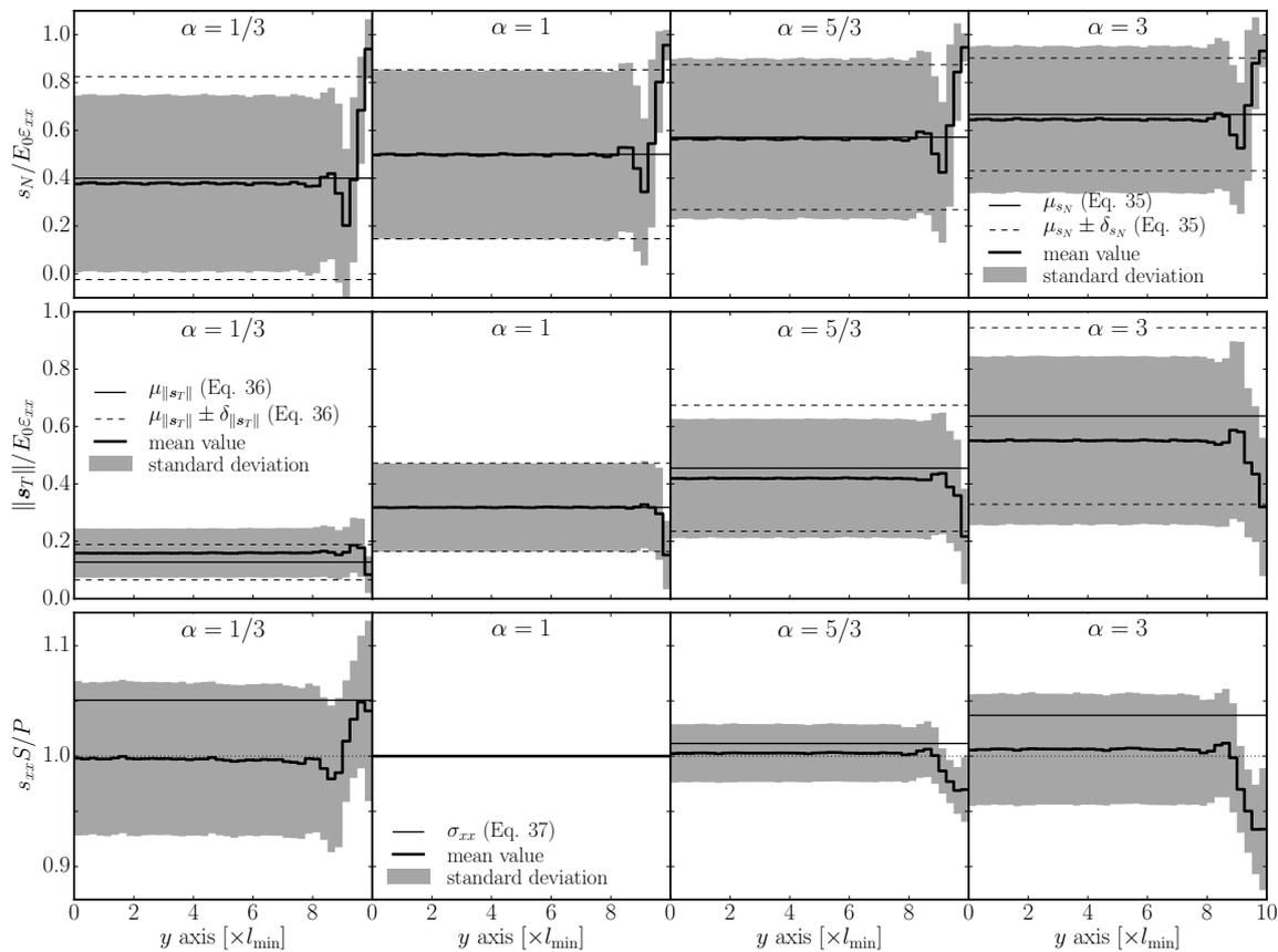
**Figure 8.** Average and standard deviation of normal stress ( $s_N$ , first row), shear stress ( $s_T$ , second row) and tensorial stress  $s_{xx}$  (third row) calculated on a half cross section under tensile loading; 2D model.
