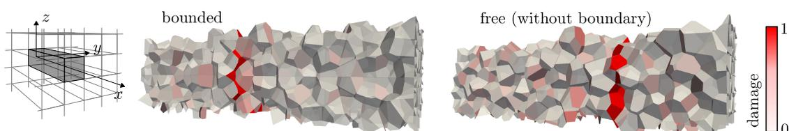
**Figure 10.** right: sketch of the periodic space; right: Damage in a 3D periodic model loaded in tension along the  $x$ -axis with and without a boundary.
