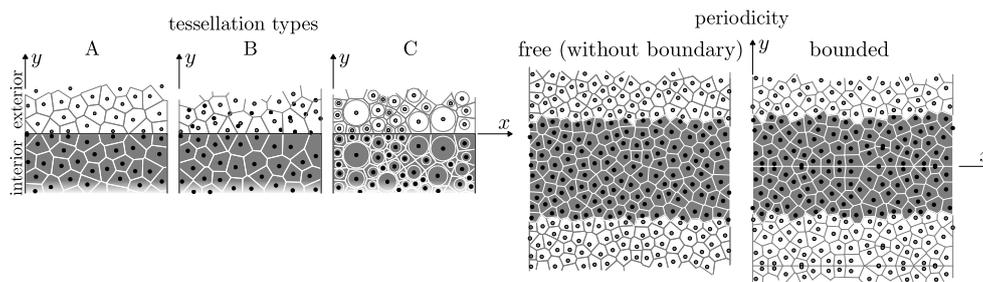
**Figure 2.** left: different tessellation types in the boundary region; right: 2D sketch of periodic structure with and without a boundary.
