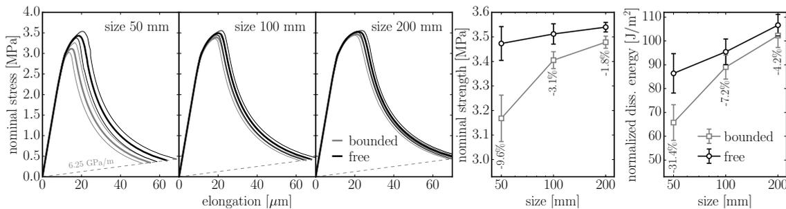
**Figure 11.** left: averaged responses of an elastically uniform periodic 3D model ( $\alpha = 1.0$ ) loaded in pure tension. Models with boundaries (*bounded*) and without boundaries (*free*) of different size are compared; right: comparison of strength and dissipated energy.
