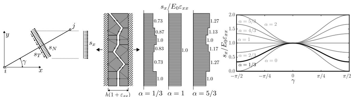
**Figure 4.** left: one element inclined by  $\gamma$  with normal and tangential stress projected into the  $x$ -direction; center: simple structure strained in the  $x$ -direction with normalized stress  $s_x$  for three different  $\alpha$  parameters; right: dependence of  $s_x$  on  $\gamma$ —Equation (7).
