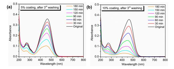
**Figure S5.** Absorption spectra of MO in presence of cashmere fabric with (a) 5% and (b) 10% TiO<sub>2</sub> nano-coating after the 3rd washing.
