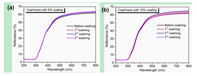
**Figure S6.** UV-vis diffuse reflectance of cashmere with (**a**) 5% TiO<sub>2</sub> coating and (**b**) 10% TiO<sub>2</sub> coating after washing.
