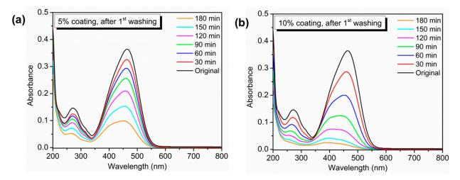
**Figure S3.** Absorption spectra of MO in presence of cashmere fabrics with (a) 5% and (b) 10% TiO<sub>2</sub> nano-coatings after the 1st washing.
