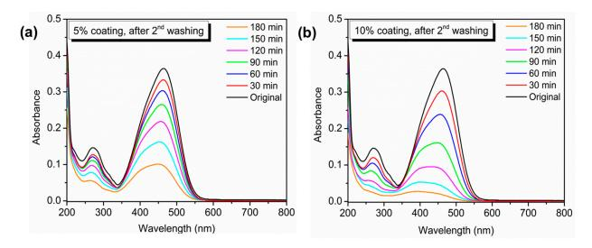
**Figure S4.** Absorption spectra of MO in presence of cashmere fabric with (a) 5% and (b) 10% TiO<sub>2</sub> nano-coating after the 2nd washing.
