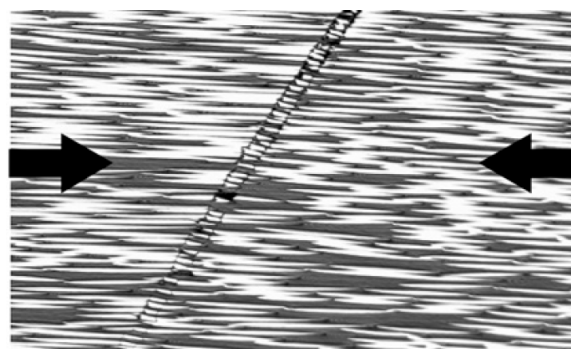
Figure 6. Example of kink band formation in a carbon fibre/epoxy specimen (reprinted from Laffan et al. [100], with permission from Elsevier).
