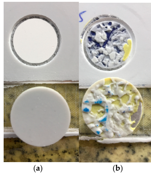
Figure 24. Pull-off strength testing of specimen laminates used for LEP coating adhesion: (a) adhesive failure with no-primer intermediate layer application; (b) cohesive failure with primer application (the dolly adhesive effect can also be observed).
