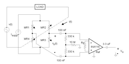
Figure 7. Signal conditioning electronics of the current channel.
