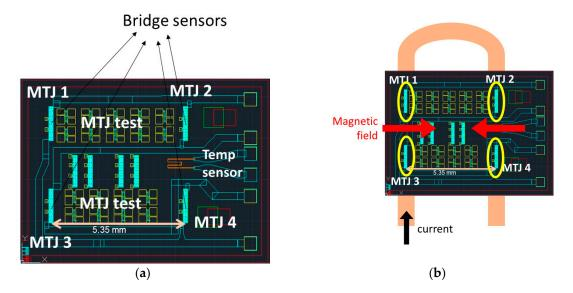
**Figure 1.** (a) Design of the chip with the four magnetic tunnel junction (MTJ) sensors connected in the Wheatstone bridge, several MTJ test elements, and a temperature sensor [30]; (b) Operation schematics, showing the opposite field created at each pair of MTJ elements by the U-shaped test current line.
