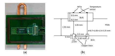
**Figure 4.** (a) Printed circuit board (PCB) including the complete tunneling magnetoresistance (TMR) transducer and the U-shaped copper current trace; (b) Cross-section schematics of the geometry used for this device, showing the copper trace dimensions as well as the sensor to trace distance.
