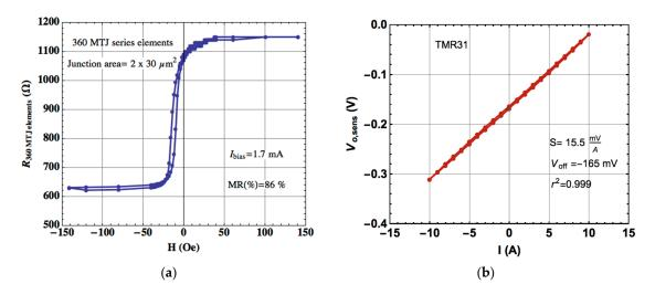
**Figure 3.** (a) R-H (resistance-to-field) characteristic of a series of 360 MTJ elements in association; (b) V-I (voltage-to-current) characteristic of the current sensor TMR31 (Wheatstone bridge) at room temperature.
