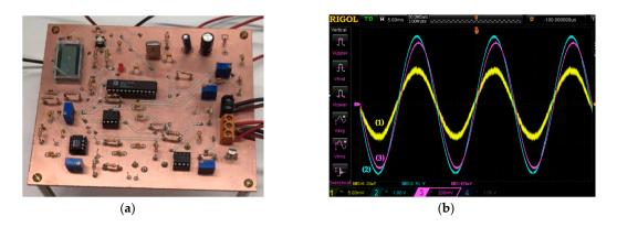
**Figure 12.** (a) Prototype energy meter implementation; (b) Experimental waveforms: (1) TMR sensor output voltage (6.2 mV<sub>rms</sub>); (2) Conditioned output voltage (2.51 V<sub>rms</sub>); (3) Electrical current through resistive load (4.59 A<sub>rms</sub> and P<sub>load</sub> = 1000 W).
