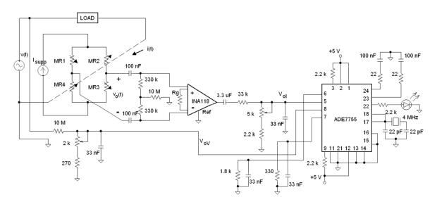
Figure 11. Whole schematic circuit that constitutes the TMR-based energy meter.
