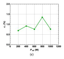
**Figure 10.** (a) Comparison between the experimental (TMR wattmeter) and reference wattmeter (2551 Xitron) active powers; (b) Actual active power vs. TMR wattmeter number of counts; (c) Obtained experimental relative uncertainty.
