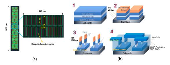
**Figure 2.** (a) Detail of the Wheatstone bridge resistances, which include 360 individual  $2 \times 30 \ \mu\text{m}^2 \text{ MTJ}$  elements connected in series; (b) Description of the microfabrication process to connect the  $2 \times 30 \ \mu\text{m}^2$  elements in series.
