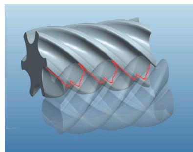
**Figure 5.** Contact line formed between rotors.
