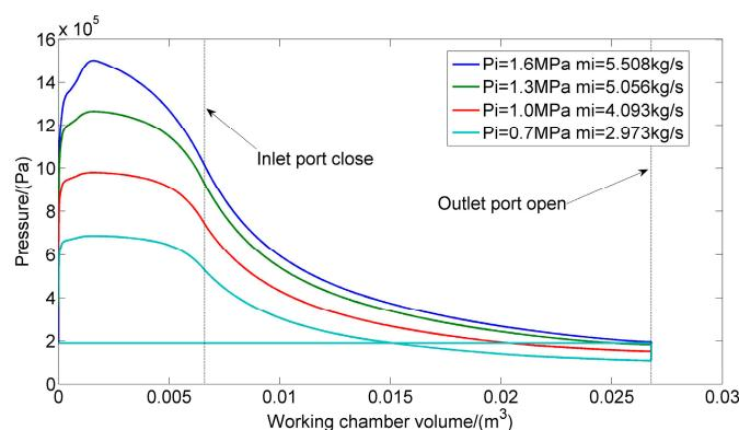
**Figure 13.** P-V diagram for different inlet pressure ( $P_o = 0.19$  Mpa,  $n = 2400$  rpm).
