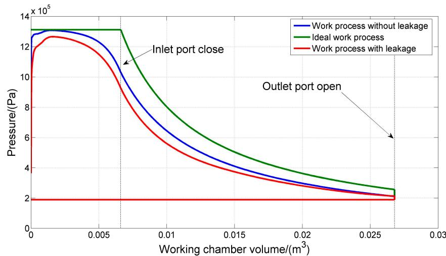
**Figure 8.** P-V diagram of ideal and simulated work process ( $P_i = 1.3 \text{ MPa}$ ,  $T_i = 192 \text{ }^\circ\text{C}$ ,  $m_t = 20 \text{ t/h}$ ,  $P_o = 0.19 \text{ MPa}$ ,  $n = 2400 \text{ rpm}$ ).
