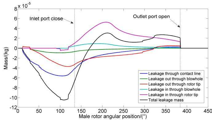
**Figure 10.** Simulated leakage mass over the rotation angle of the male rotor during the expansion process ( $P_i = 1.3 \text{ MPa}$ ,  $T_i = 192^\circ\text{C}$ ,  $m_t = 20 \text{ t/h}$ ,  $P_o = 0.19 \text{ Mpa}$ ,  $n = 2400 \text{ rpm}$ ).
