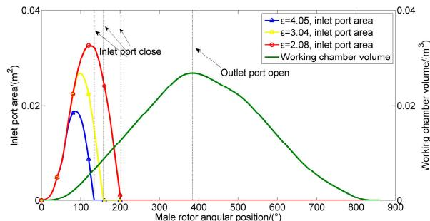
**Figure 4.** Inlet area and volume curve of the screw expander.
