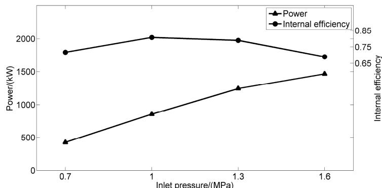
**Figure 14.** Internal efficiency and power for different inlet pressure ( $P_o = 0.19$  Mpa,  $n = 2400$  rpm).
