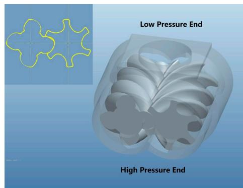
**Figure 3.** 3D geometry model and rotor profile.
