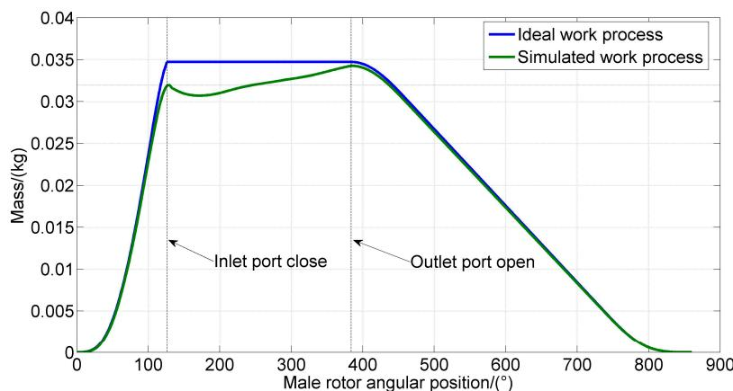
**Figure 9.** m-θ diagram of ideal and simulated work process ( $P_i = 1.3 \text{ MPa}$ ,  $T_i = 192 \text{ }^\circ\text{C}$ ,  $m_t = 20 \text{ t/h}$ ,  $P_o = 0.19 \text{ MPa}$ ,  $n = 2400 \text{ rpm}$ ).
