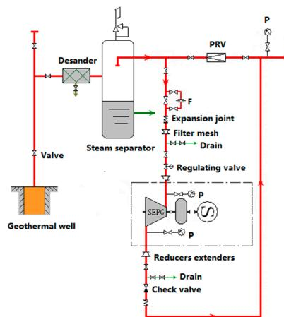
**Figure 2.** Schematic drawing of the screw expander power generation unit.
