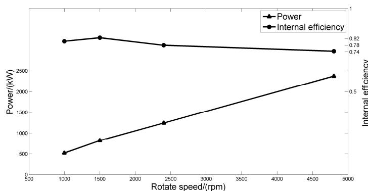
**Figure 12.** Internal efficiency and power for different rotate speed ( $P_i = 1.3 \text{ MPa}$ ,  $T_i = 192^\circ\text{C}$ ,  $P_o = 0.19 \text{ Mpa}$ ).
