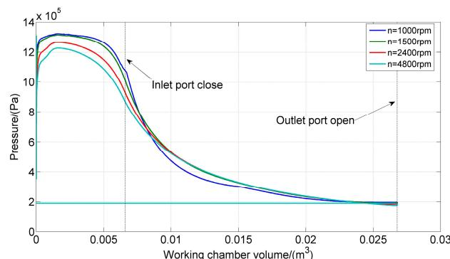
**Figure 11.** P-V diagram for different rotate speed ( $P_i = 1.3 \text{ MPa}$ ,  $T_i = 192^\circ\text{C}$ ,  $P_o = 0.19 \text{ Mpa}$ ).
