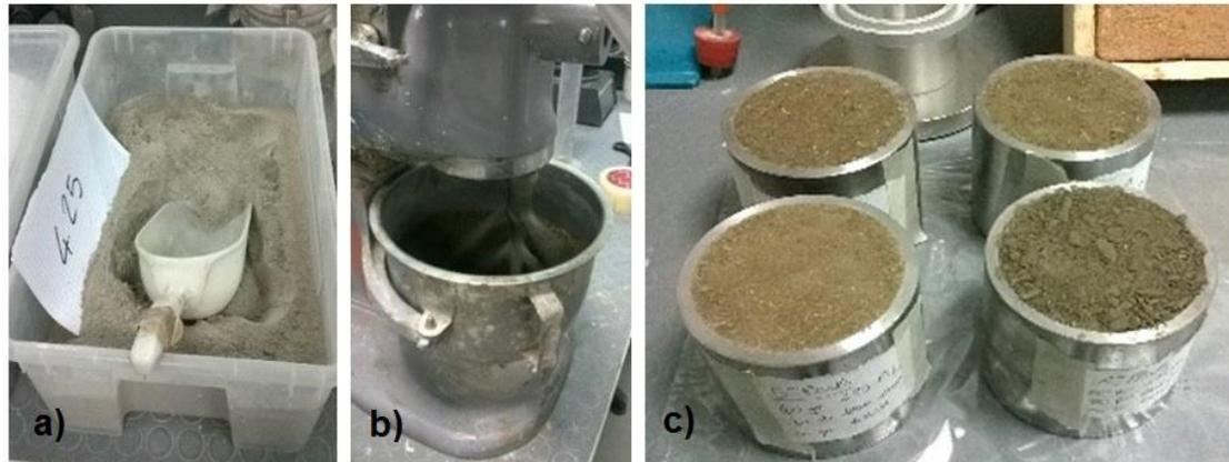
**Figure 5.** Mixing procedure of the mineralization process (a) Portland cement 4.25; (b) The material mixer; (c) The prepared samples and the moulds.
