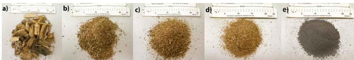
Figure 4. Pictures of the type 1 unbound material (a) 20–30 mm; (b) 4 mm; (c) 2 mm; (d) 1 mm; (e) lignin flour.
