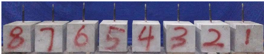
Figure 8. Completed sandstone specimens ready for hydraulic fracturing testing.
